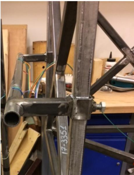
Figure 3.1: Clamping system of bumper on module
