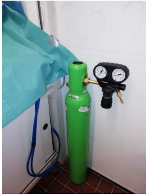
Figure 13. Bottle with 95% standard air and 5% carbon dioxide gas.
