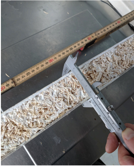
Image 5.21: Assessing thickness with analogue calliper
