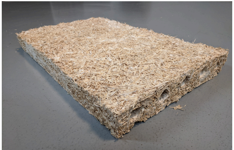
Image 6.29 - 6.33: The various steps of prototyping a hollow core slap
