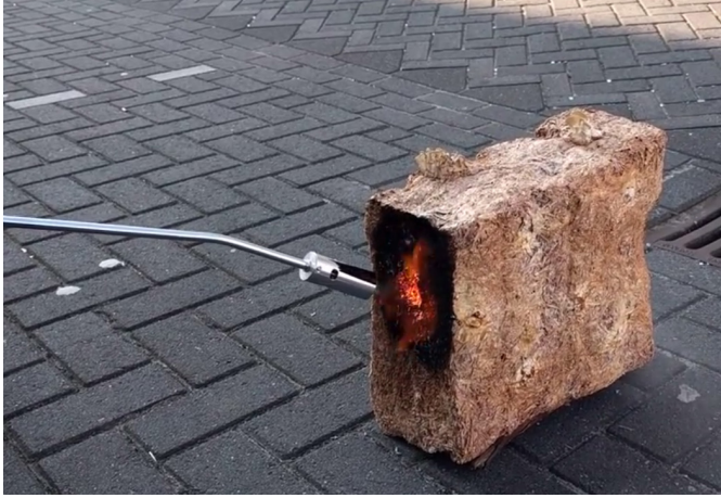
Image 2.19 & 20 DIY fire tests with mycelium-based composites
