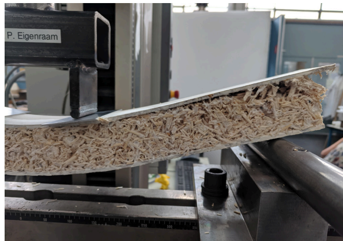
Image 5.40: Delamination showing at end of sample
