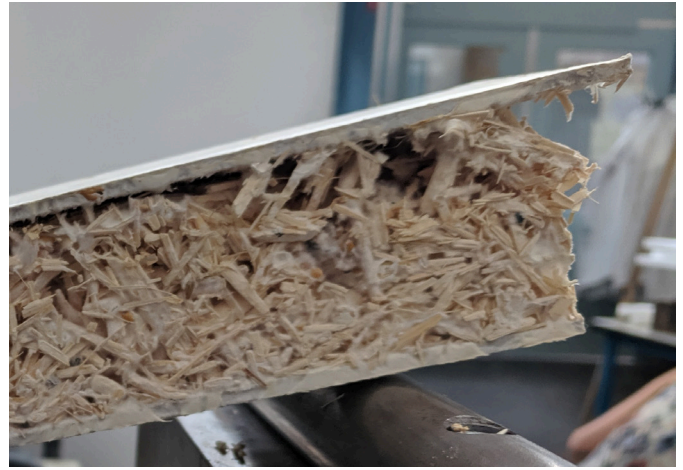
Image 5.72: Delamination causing peltruding ends
