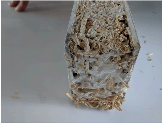
Image 5.79: Sample ends grew less due to dehydration
