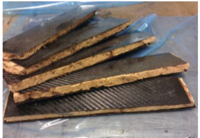
Image 4.09: Sandwich panel from carbon fibre and MBC by Travaglini (2014)
