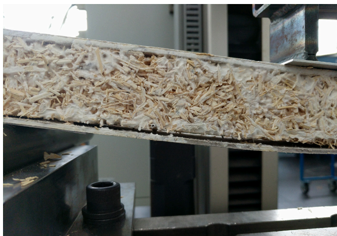
Image 5.41: Cavity between core and bottom sheet
