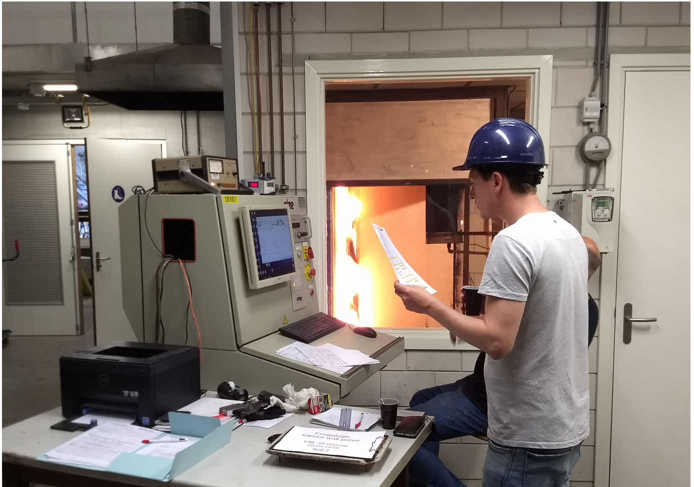
Image 2.50: Single Burning Item (SBI) test at Efectis Nederland
