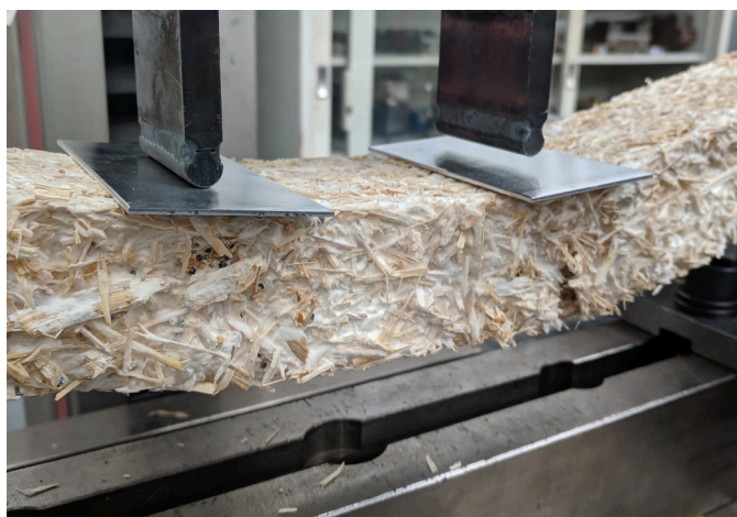
Image 5.39: Asymmetrical crack in sample 4
