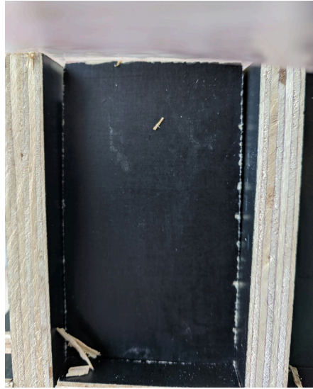
Image 5.22: Poorly made end of mould causing dehydration
