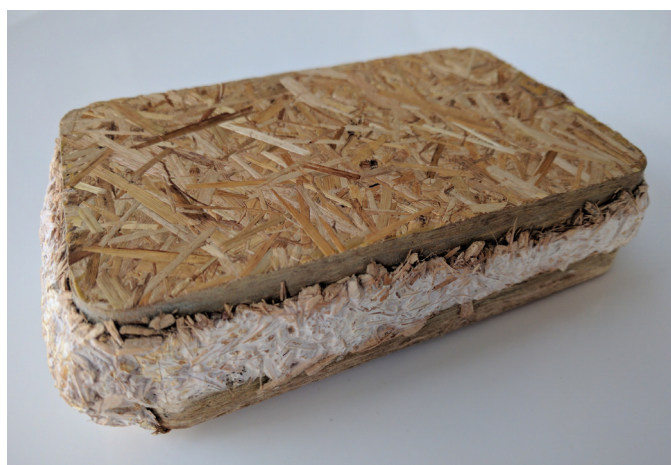
Image 1.06: Fungal sandwich panel, proof of concept
