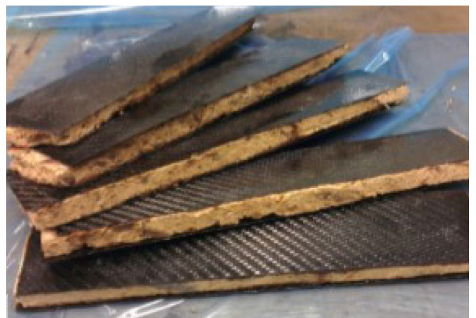
Image 2.47: Sandwich panel from carbon fibre and MBC by Travaglini (2014)
