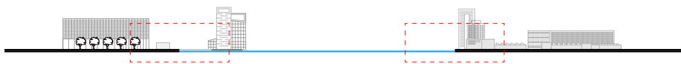
Figure 6.15: The design envelope for the landings of the bridge and the quays (own illustration)
