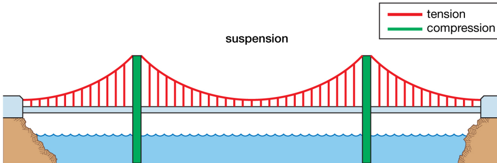
Figure 5.16: The tension and compression indicated in red and green show the structural principle of a suspension bridge (Encyclopædia Britannica, Inc.)
