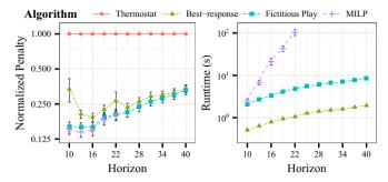
**Figure 1.** Algorithm performance for increasing horizon: policy quality normalized to the thermostat policy (left), and wall-clock computation time (right). Both plots on a log scale, lower values are better.
