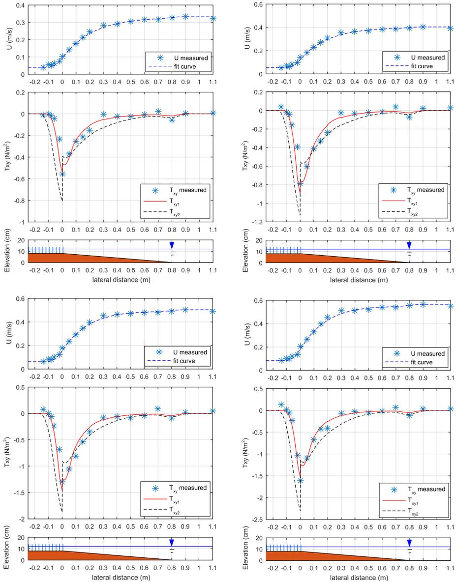
Figure B.5: Profile of mean streamwise velocity, and the comparison of modelled transverse shear stress according to the eddy viscosity model of this study  $T_{xy1}$ , in cases Bs1, Bs2, Bs3, Bs4 (left upper panel, right upper panel, left lower panel, right lower panel, respectively), and  $T_{xy2}$  [White and Nepf, 2008].
