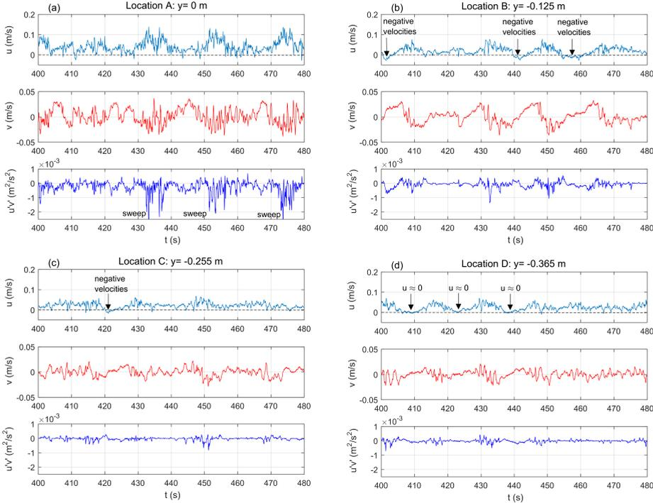
Figure 3.10: Time series of streamline velocity  $u$  (solid line), lateral velocity  $v$  (dash line) and the shear stress ( $u'v'$ ) ( $10^{-3}$ ) at locations A:  $y=0$  m (a) ; B:  $y=-0.125$  m (b) ; C:  $y=-0.255$  m (c) and D:  $y=-0.365$  m (d) in case of dense vegetation, 50 cm floodplain width, discharge =45 l/s and water level =12 cm.
