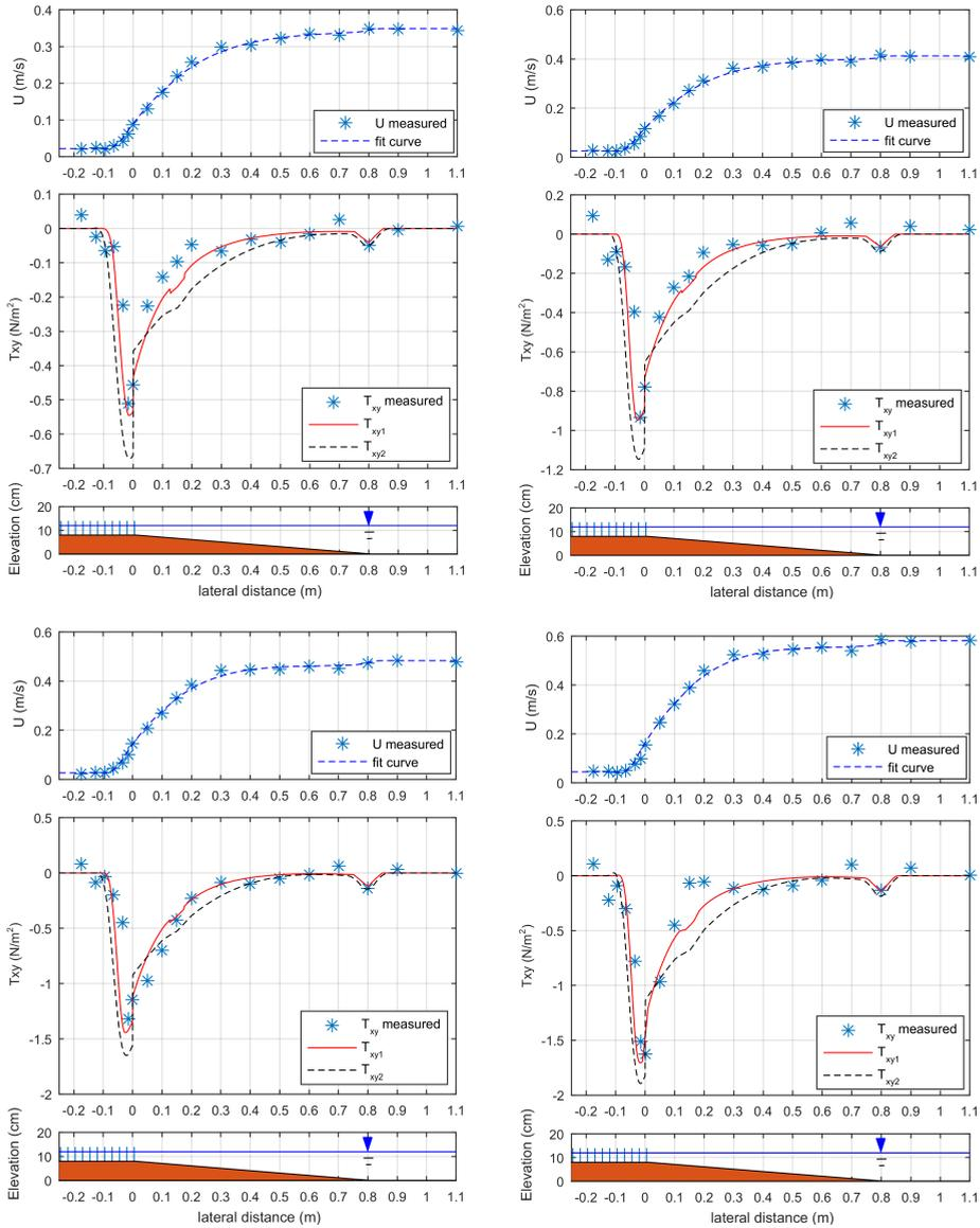
Figure B.2: Profile of mean streamwise velocity, and the comparison of modelled transverse shear stress according to the eddy viscosity model of this study  $T_{xy1}$ , in cases Bd1, Bd2, Bd3, Bd4 (left upper panel, right upper panel, left lower panel, right lower panel, respectively), and  $T_{xy2}$  [White and Nepf, 2008].
