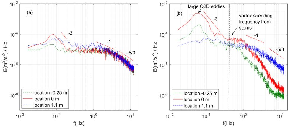
Figure 3.6: Power density spectra of lateral velocity fluctuations at different locations from the wall – No and Dense vegetation scenario, 50 cm width, discharge =45 l/s, water level =12 cm;  $y = -0.25$  m located inside the vegetation,  $y = 0$  m located at the vegetated floodplain edge,  $y = 1.1$  m location outside in the main channel.
