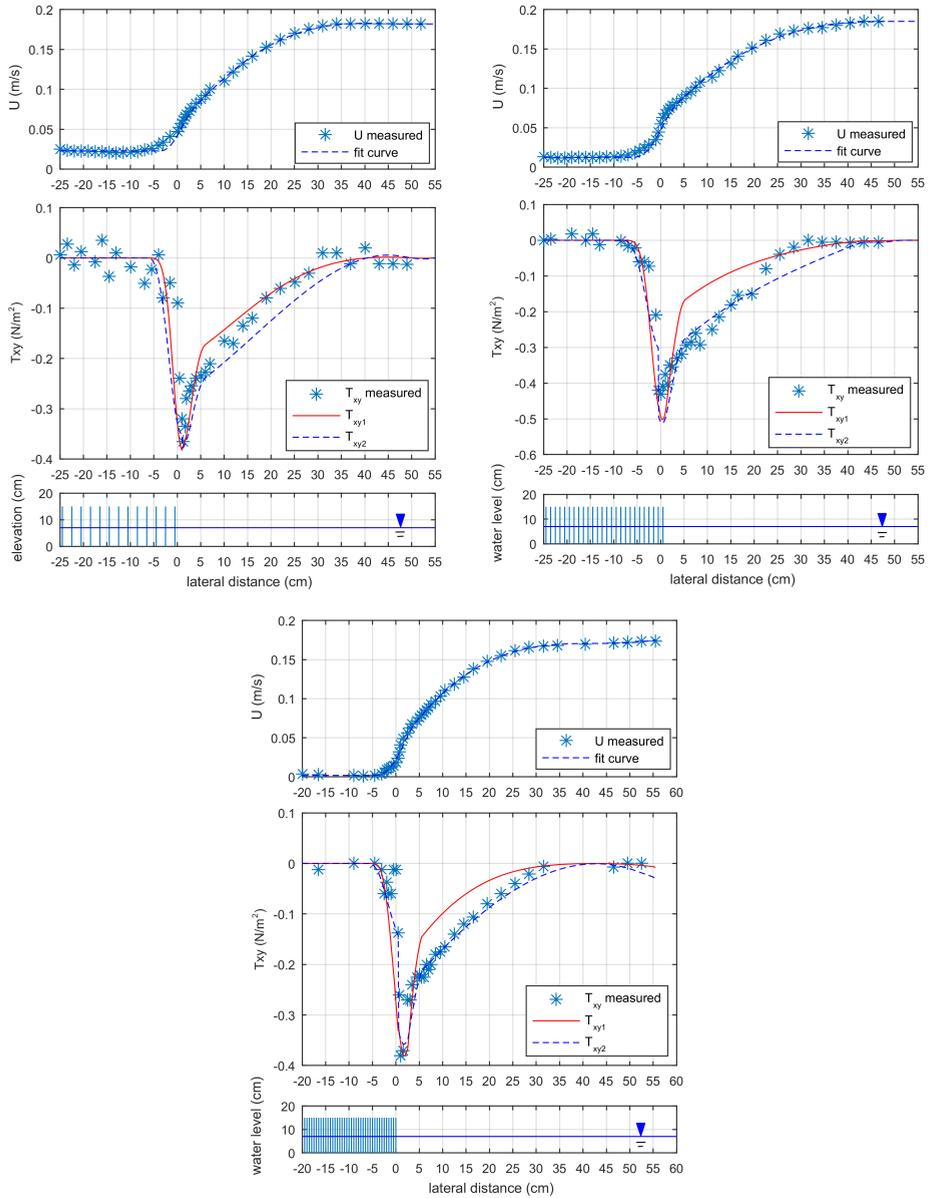
Figure B.9: Profile of mean streamwise velocity, and the comparison of modelled transverse shear stress according to the eddy viscosity model of this study  $T_{xy1}$ , in cases I, IV, VII of White and Nepf [2008] (left upper panel, right upper panel, lower panel, respectively), and  $T_{xy2}$  [White and Nepf, 2008].
