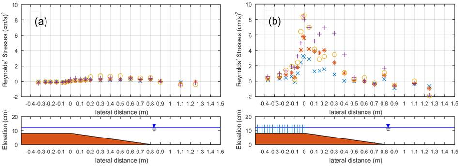
Figure 3.5: Reynolds shear stress ( $-\overline{u'v'}$ ) no cylinder cases (a) and dense cases (b), 50 cm width; different input discharge and water level. Legend qxxyy refers to a discharge of xx l/s and a water depth of yy cm. Crosses: q45h12, stars: q60h13, plusses: q80h14, circles: q80h12.
