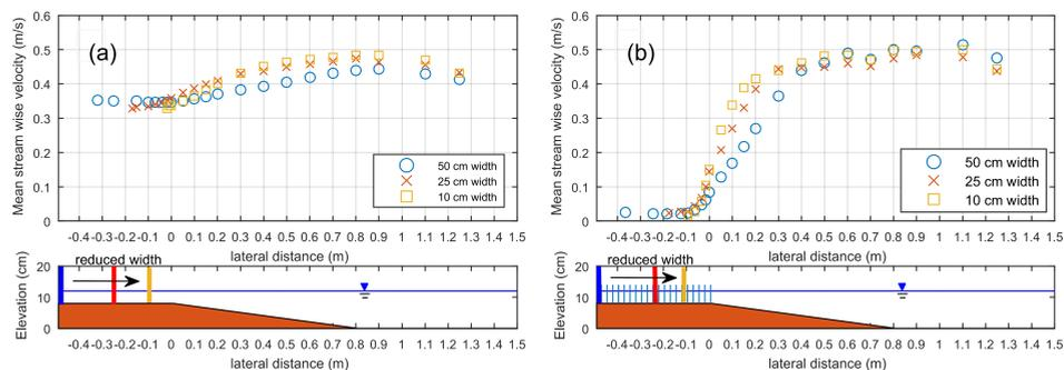
Figure 3.15: Mean streamwise velocity profile in non-vegetated floodplain scenarios and dense vegetation scenarios, discharge  $Q=80 \text{ L s}^{-1}$ , water level  $H=14 \text{ cm}$ , different floodplain widths – circles: 50 cm; crosses: 25 cm; squares: 10 cm.
