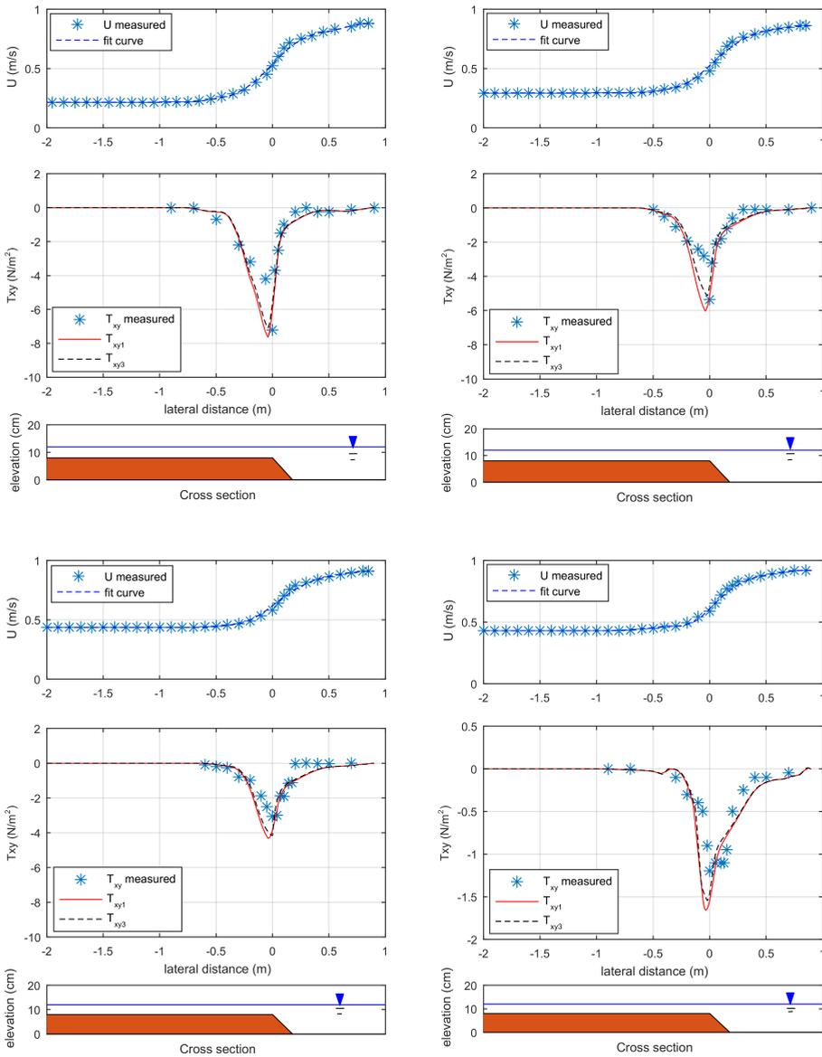
Figure B.10: Profile of mean streamwise velocity, and the comparison of modelled transverse shear stress according to the eddy viscosity model of this study  $T_{xy1}$ , in cases  $Dr = 0.11, 0.15, 0.20$  and  $0.25$  (left upper panel, right upper panel, left lower panel, right lower panel, respectively) of Lambert and Sellin [1996] and Ervine et al. [2000], and  $T_{xy3}$  [van Prooijen et al., 2005].
