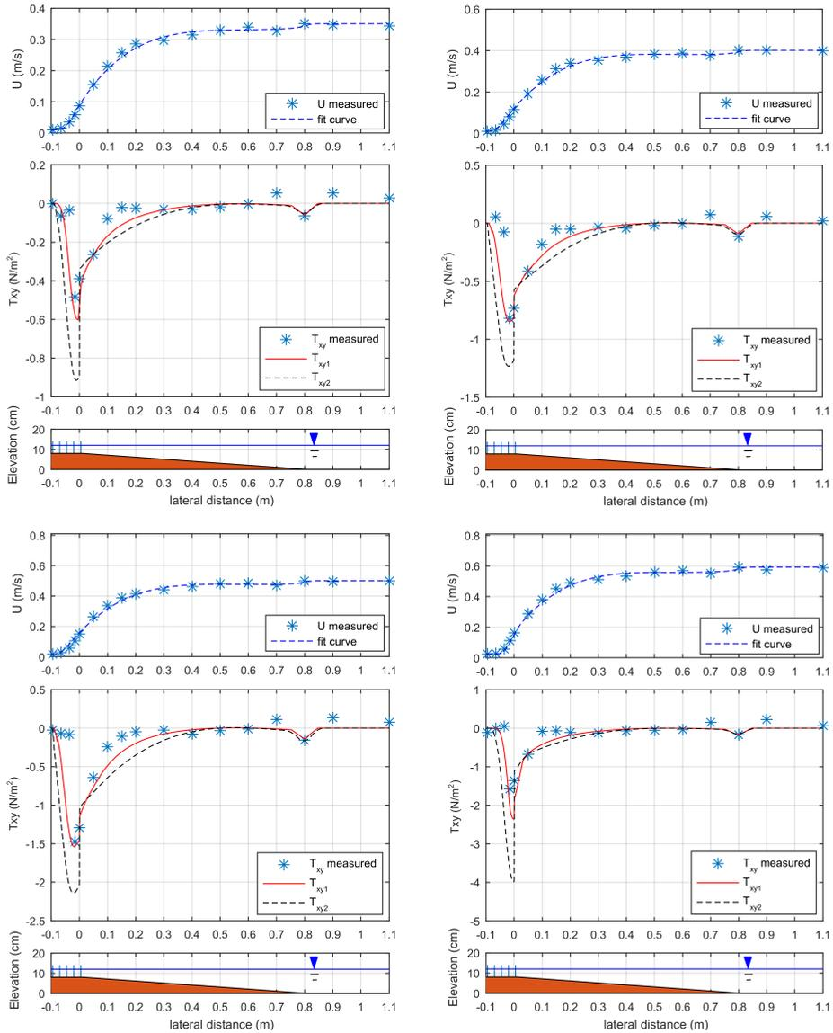
Figure B.3: Profile of mean streamwise velocity, and the comparison of modelled transverse shear stress according to the eddy viscosity model of this study  $T_{xy1}$ , in cases Cd1, Cd2, Cd3, Cd4 (left upper panel, right upper panel, left lower panel, right lower panel, respectively), and  $T_{xy2}$  [White and Nepf, 2008].
