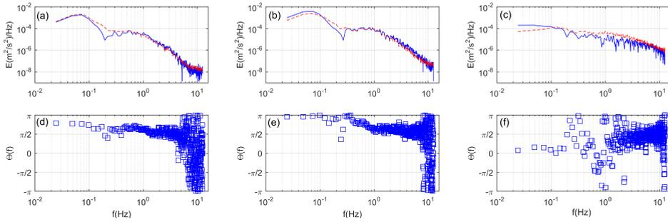
Figure 3.7: Dense case – Cross Power density spectral, case 50 cm width, and discharge = 45 l/s, water level = 12 cm: location  $y = -0.065$  m (inside the vegetation) (a), location  $y = 0$  m (at the edge) (b) and  $y = 1.1$  m (in the main channel) (c) - Blue line ( $u'v'$  spectrum); Red line ( $v'v'$  spectrum). The phase relation between  $u'$  and  $v'$ : location  $y = -0.065$  m (d), location  $y = 0$  m (e) and  $y = 1.1$  m (f).
