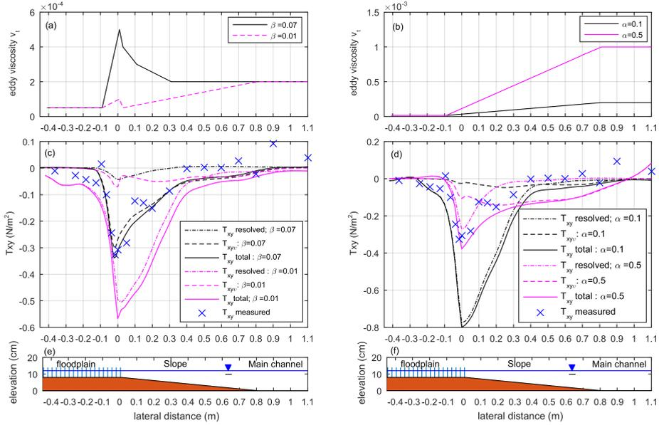
Figure 5.8: Sensitive analysis of the  $\beta$  and  $\alpha$  in terms of the transverse shear stresses. Transverse shear stresses were over predicted when  $\beta$  was reduced from 0.07 to 0.01 (a) and are in fairly agreement with the measured data when  $\alpha$  was increased from 0.1 to 0.5 (b).
