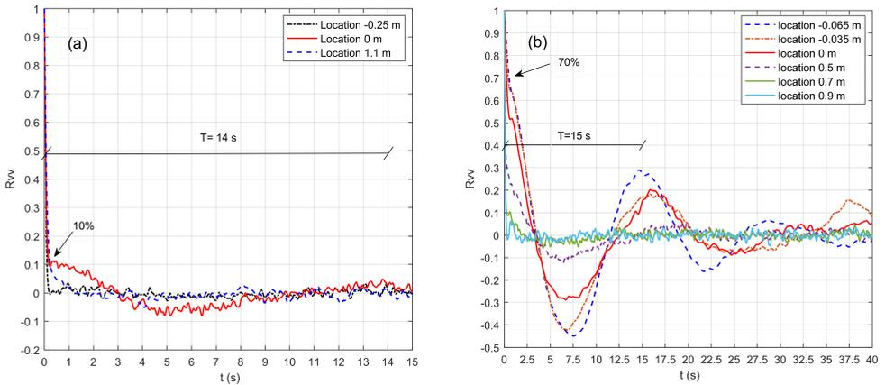
Figure 3.8: Autocorrelation function  $R_{vw}$ , 50 cm width, discharge =45 l/s, water level =12 cm; (a) No vegetation, (b) Dense vegetation.
