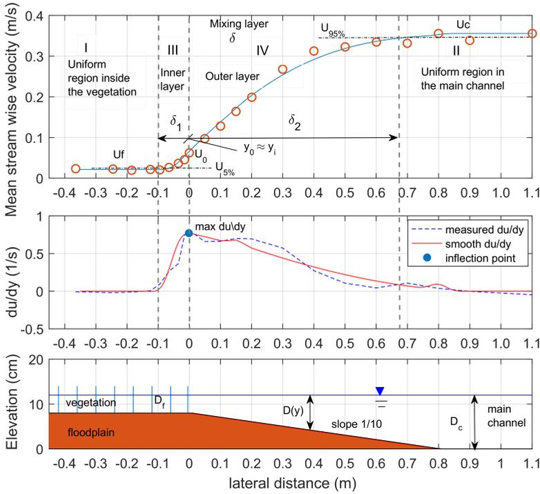
Figure 4.7: Representative mean streamwise velocity profile in cases with the consideration of vegetation. The most interesting region is the mixing layer, including the penetration ( $\delta_1$ ) or inner layer part and the outer layer part ( $\delta_2$ ).  $Q=45 \text{ L s}^{-1}$ ,  $H=12 \text{ cm}$ , width= 50 cm.
