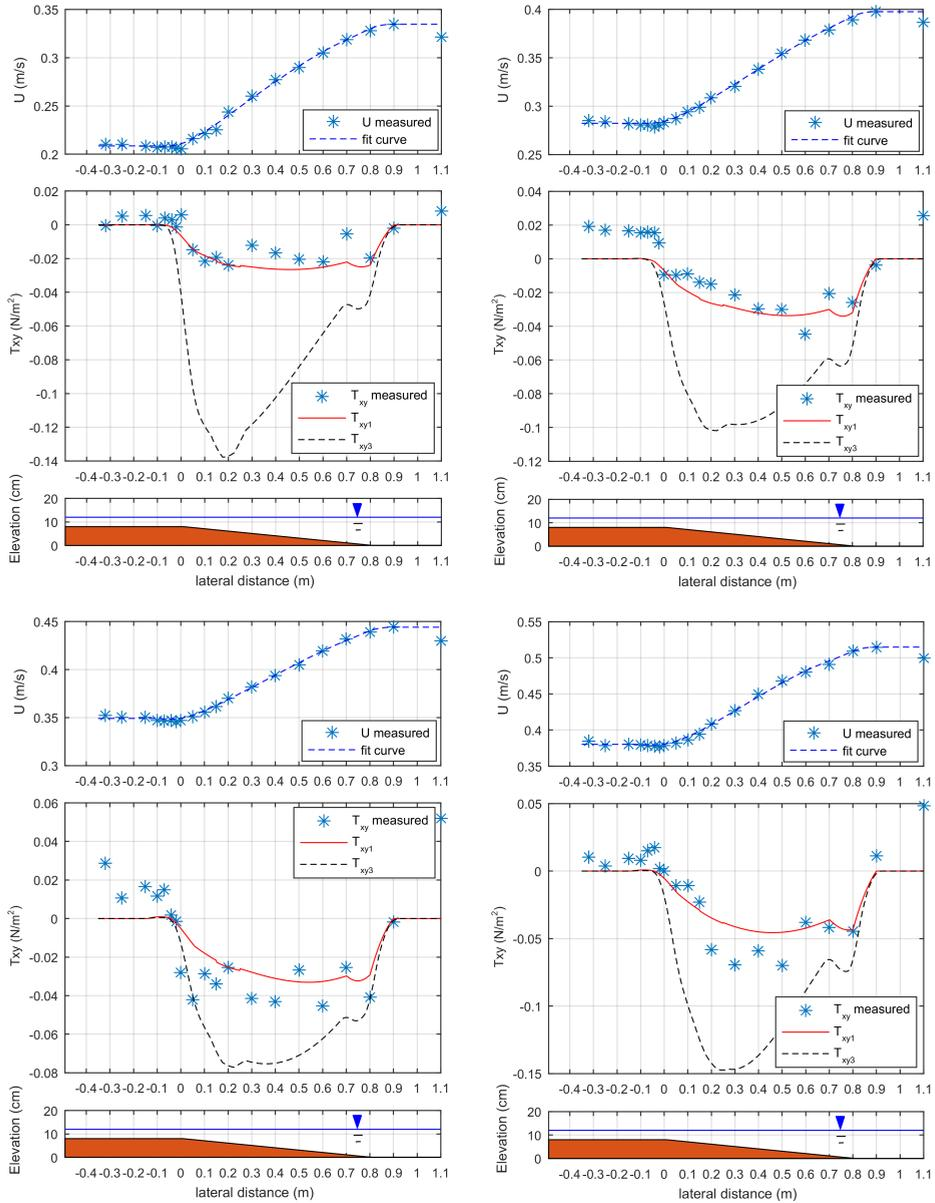
Figure B.7: Profile of mean streamwise velocity, and the comparison of modelled transverse shear stress according to the eddy viscosity model of this study  $T_{xy1}$ , in cases An1, An2, An3, An4 (left upper panel, right upper panel, left lower panel, right lower panel, respectively), and  $T_{xy3}$  [van Prooijen et al, 2005].
