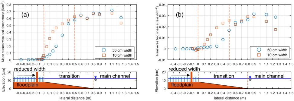
Figure 3.20: Streamwise bed shear stress comparison(a) and transverse bed shear stress comparison(b) in scenarios of 50 cm and 10 cm floodplain width, discharge  $Q = 80\text{Ls}^{-1}$ , water level  $H = 14\text{ cm}$ . The positive values of the transverse bed shear stress indicate that it is directed away from the floodplain.
