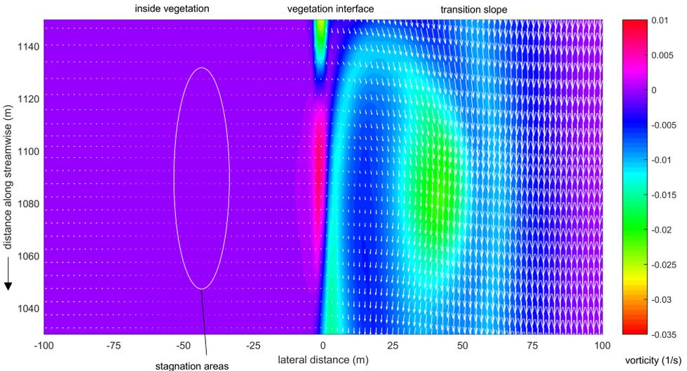
Figure 5.13: The field of vorticity and the corresponding velocity field reveals and presence of the LHCs and its effects on the flow field at real scale.
