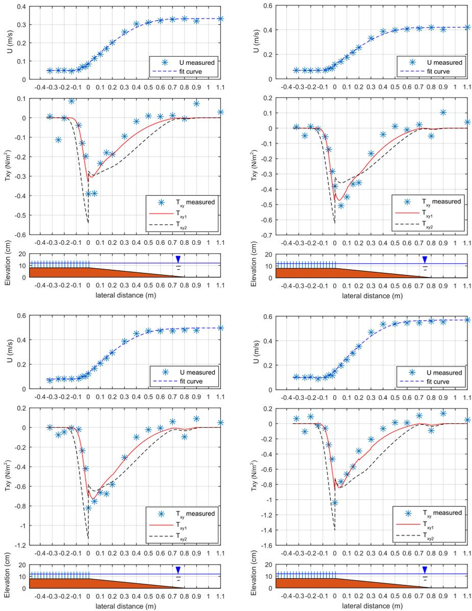
Figure B.4: Profile of mean streamwise velocity, and the comparison of modelled transverse shear stress according to the eddy viscosity model of this study  $T_{xy1}$ , in cases As1, As2, As3, As4 (left upper panel, right upper panel, left lower panel, right lower panel, respectively), and  $T_{xy2}$  [White and Nepf, 2008].
