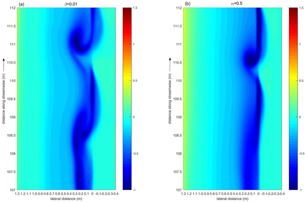
Figure 5.9: Representative vorticity resolved by the model in which the eddy viscosity was determined by the hybrid eddy viscosity model (left panel,  $\beta = 0.01$ ), and by Elder formulation (right panel  $\alpha = 0.5$ ).
