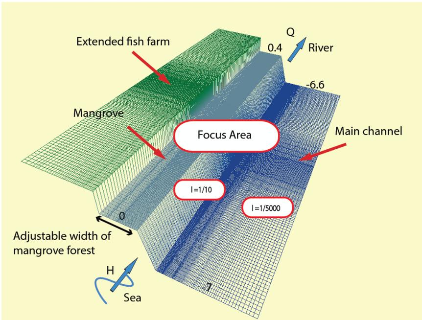
Figure 2.7: Tieu - 3D schematised model. The model includes a main river and a floodplain. It covers the first two kilometers length from the river mouth, and half of the estuarine width.
