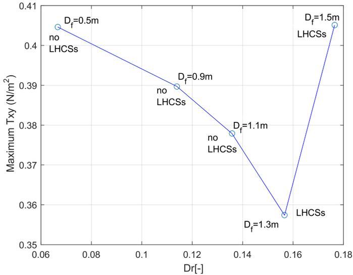
Figure 5.12: The relationship between the maximum transverse shear stress, water depth and the presence of LHCs predicted by the simulations.
