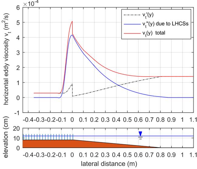
Figure 4.8: Eddy viscosity profile determined according to the hybrid eddy viscosity model and based on the measured velocity profile, in case of dense cylinder,  $Q=45\text{ L s}^{-1}$ ;  $H=12\text{ cm}$  and floodplain width  $W=50\text{ m}$ .
