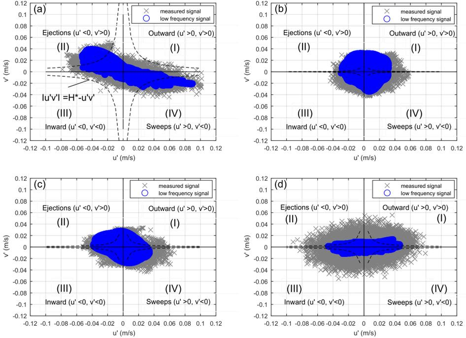
Figure 4.6: The representative distribution of  $(u', v')$  measured the low frequency signal for dense scenarios, q45h12 : at location  $y = 0$  m (at the vegetation interface),  $H = 2$  (a);  $y = -0.015$  m,  $H = 2$  (b);  $y = -0.065$  m (inside the vegetation),  $H = 2$  (c);  $y = 1.25$  m (in the main open channel),  $H = 5$  (d); The dashed lines in the figure represent hyperbolas corresponding to  $|u'v'| = H \cdot (-u'v')$ .
