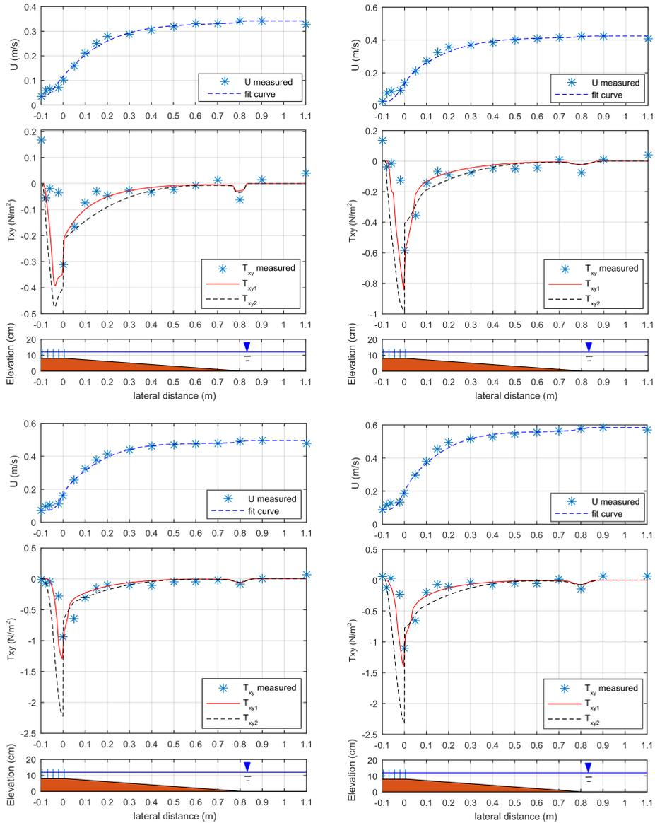
Figure B.6: Profile of mean streamwise velocity, and the comparison of modelled transverse shear stress according to the eddy viscosity model of this study  $T_{xy1}$ , in cases Cs1, Cs2, Cs3, Cs4 (left upper panel, right upper panel, left lower panel, right lower panel, respectively), and  $T_{xy2}$  [White and Nepf, 2008].
