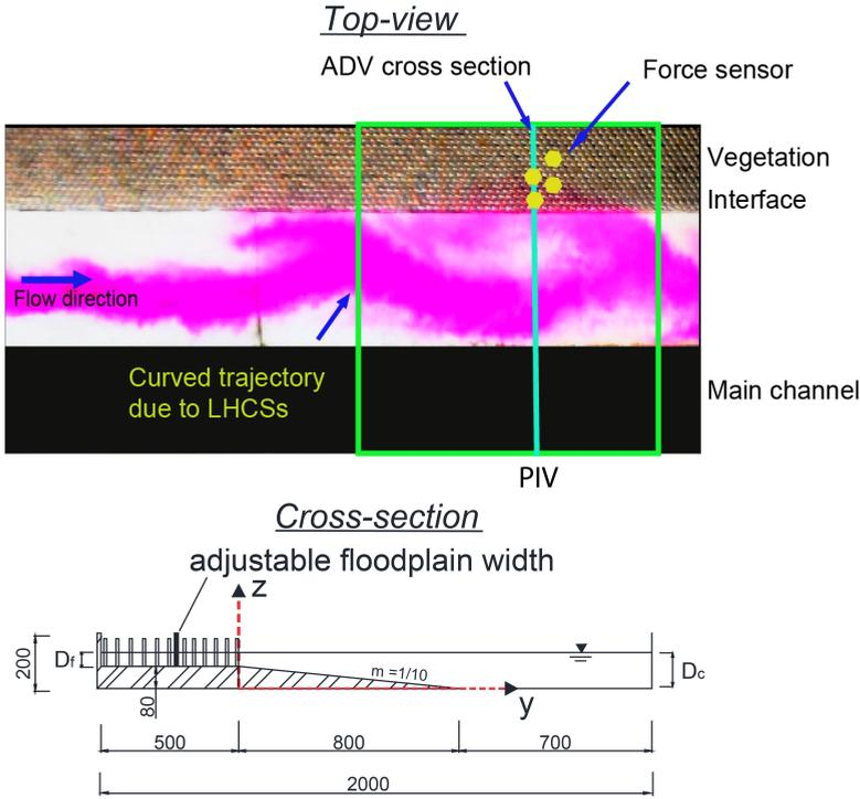
Figure 5.2: Physical model set up and measurements including top view and cross section of the experiment, dense cases, 50 cm floodplain width. The presence of LHCs can be clearly observed through color dye. It can be seen that the penetration of the dye into the cylinder array is about 20 cm which is similar to that in Figure 3.14: sparse case, 25 cm floodplain width. The similarity between the shear-layer dynamics of sparse and dense cases can also be seen in Figure A.1 in the appendix.
