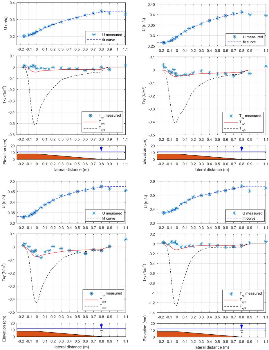
Figure B.8: Profile of mean streamwise velocity, and the comparison of modelled transverse shear stress according to the eddy viscosity model of this study  $T_{xy1}$ , in cases Bn1, Bn2, Bn3, Bn4 (left upper panel, right upper panel, left lower panel, right lower panel, respectively), and  $T_{xy3}$  [van Prooijen et al, 2005].
