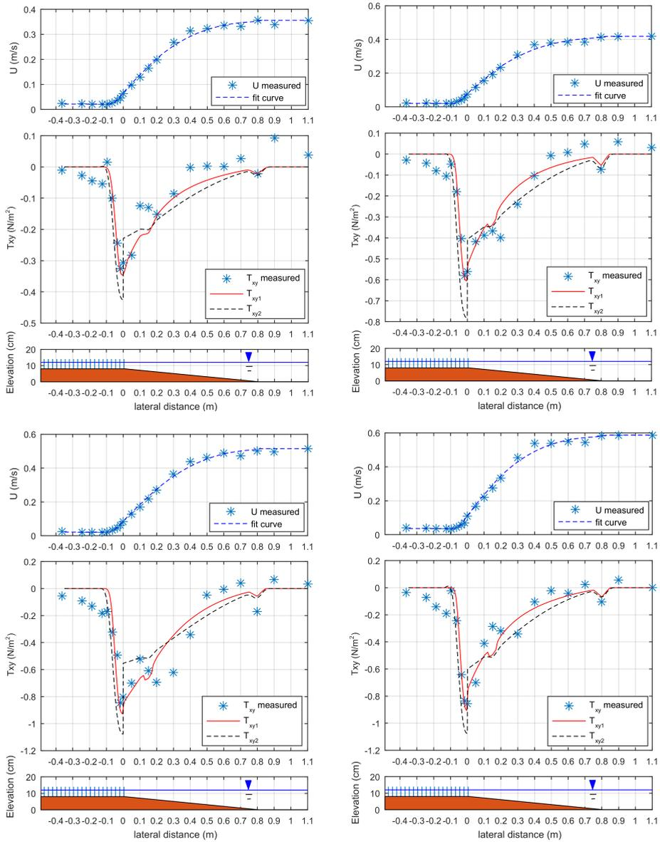
Figure B.1: Profile of mean streamwise velocity, and the comparison of modelled transverse shear stress according to the eddy viscosity model of this study  $T_{xy1}$ , in cases Ad1, Ad2, Ad3, Ad4 (left upper panel, right upper panel, left lower panel, right lower panel, respectively), and  $T_{xy2}$  [White and Nepf, 2008].
