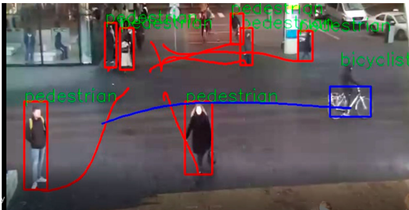
Figure 3. Sample illustration of the detection and tracking method adopted where the boxes bound the objects, and the lines retrace their trajectories.
