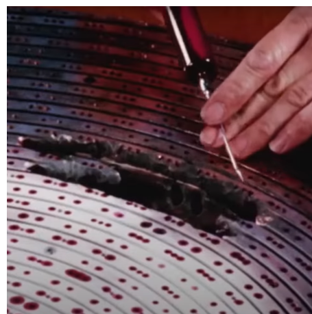
(b) Damaged F-1 injector faceplate [20]
