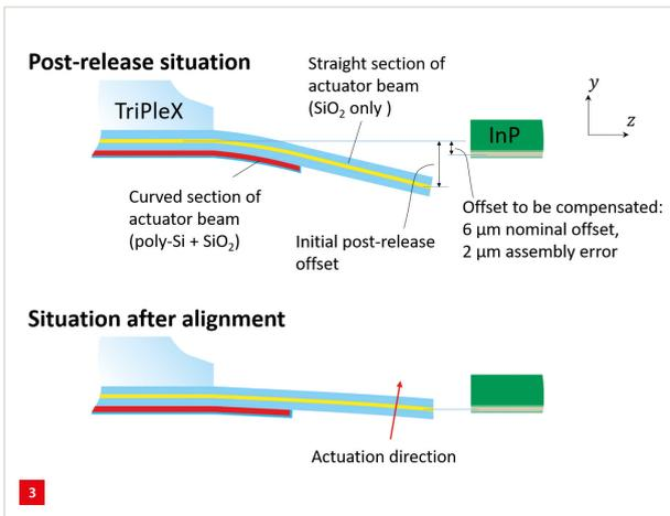
curvature, and this can be quite significant. The bimorph actuator design proposed makes intended use of the post-release deformation [8]. In this design, only a short section of the entire actuator beam is provided with poly-Si. This section will have a post-release curvature, whereas the remaining SiO<sub>2</sub>-only section of the beam is almost straight. Hence, the length of the poly-Si section is a parameter that can be used to fine-tune the initial out-of-plane position of the structure.
