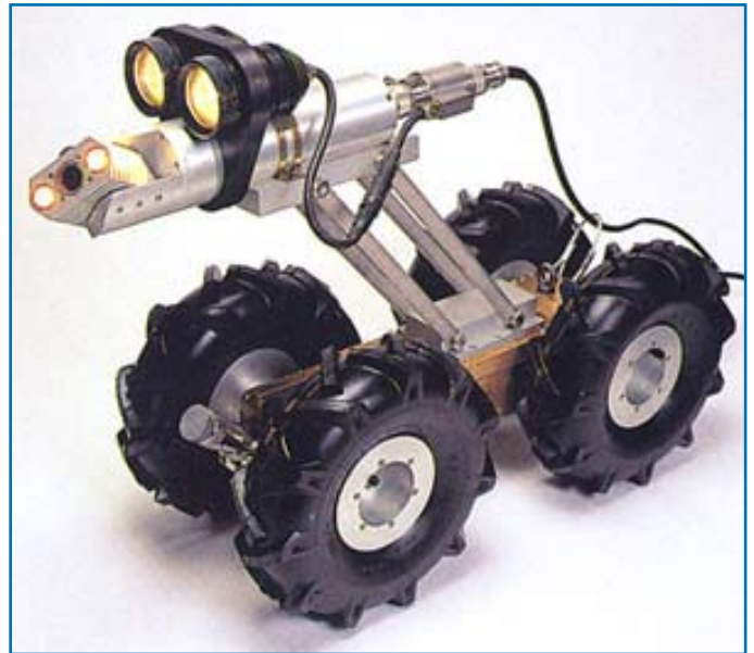
Figure 23: CCTV robot with pan-and-tilt possibility (General Utilities Northwest)
