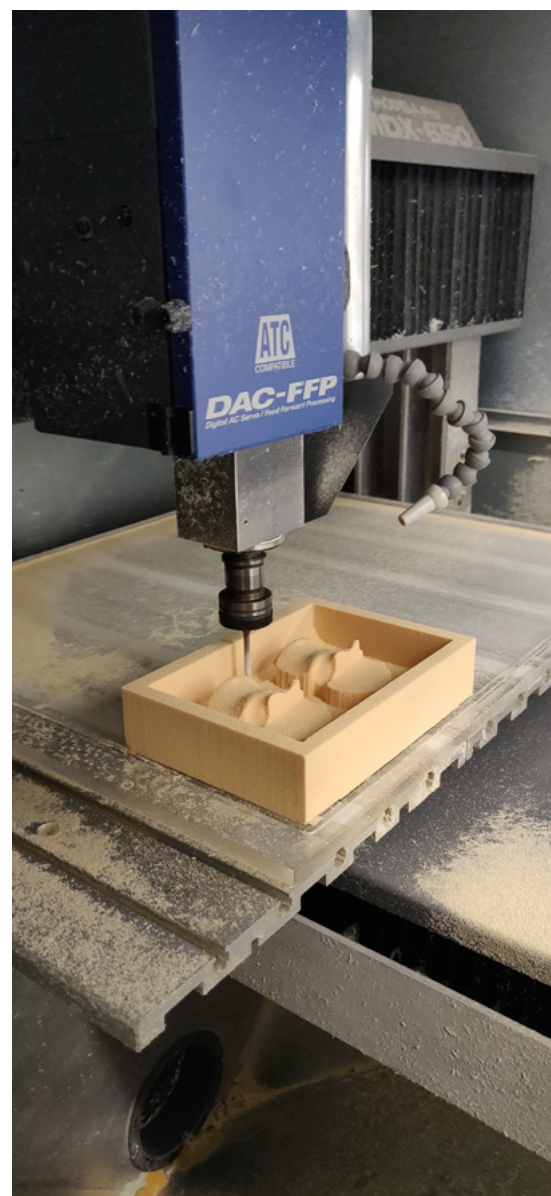
Figure 52. Milling tibial condyle out of PCF20 sawbones block
