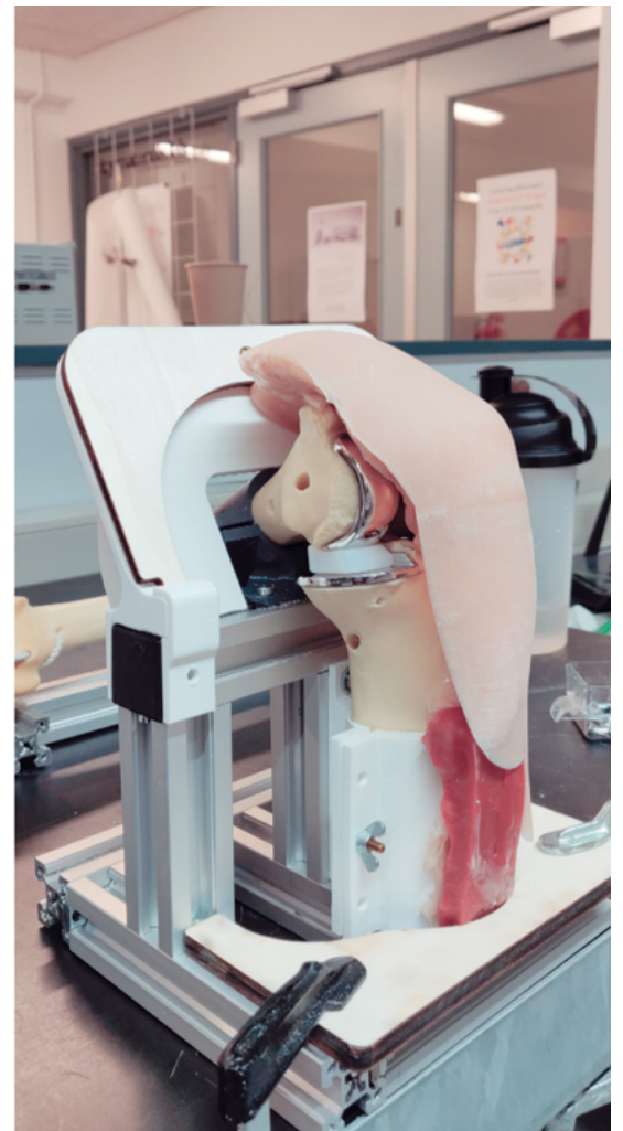
Figure 38. Silicone soft tissue around the sawbones
