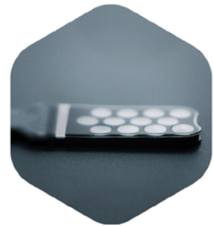
Figure 28. Micro fluidix skin inside haptX 40
