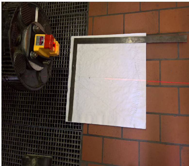
Figure 3.5: Calibration of Automated Slip angle ( \alpha ) sweep
