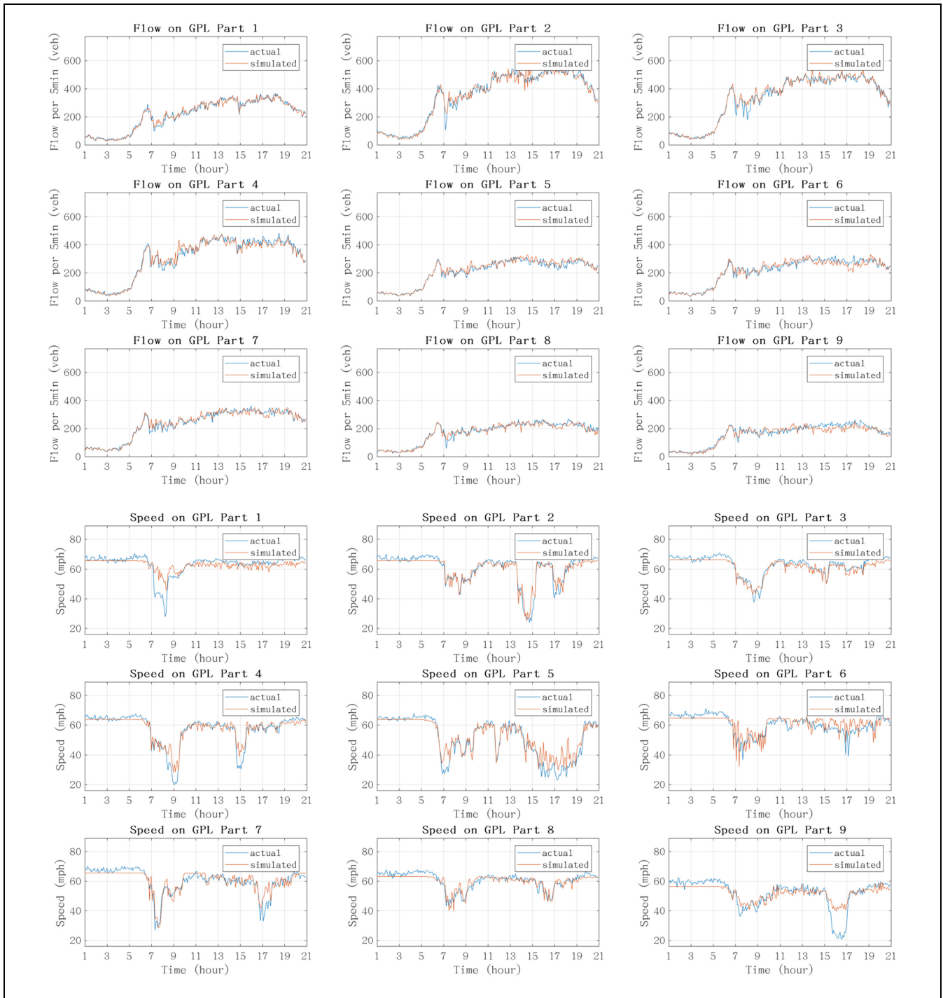
Figure 6. Comparison of actual and simulated flow and speed in GPL of WB corridor of the network: (a) flow, and (b) speed.
