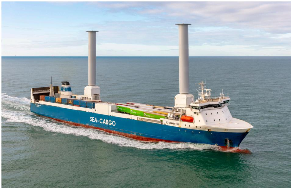
Figure 1.3: SC Connector by Sea-Cargo and Norsepower, with Flettner Rotors [26]
