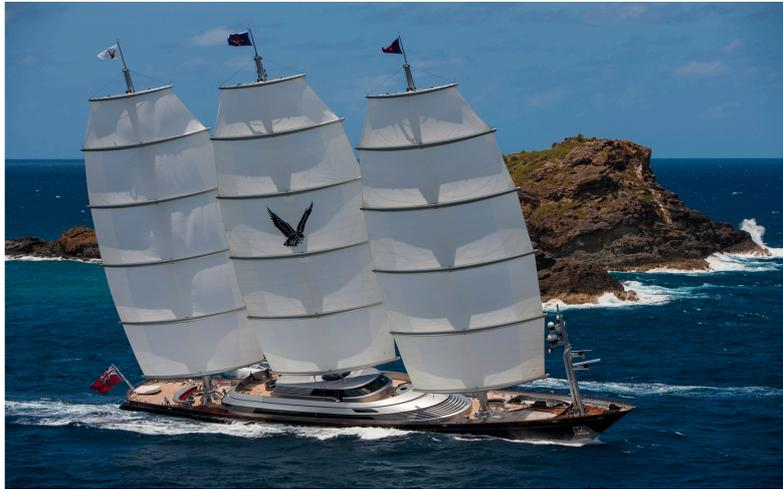
Figure 1.1: Maltese Falcon by Dykstra Naval Architects, with Dynarig Sails [8]
