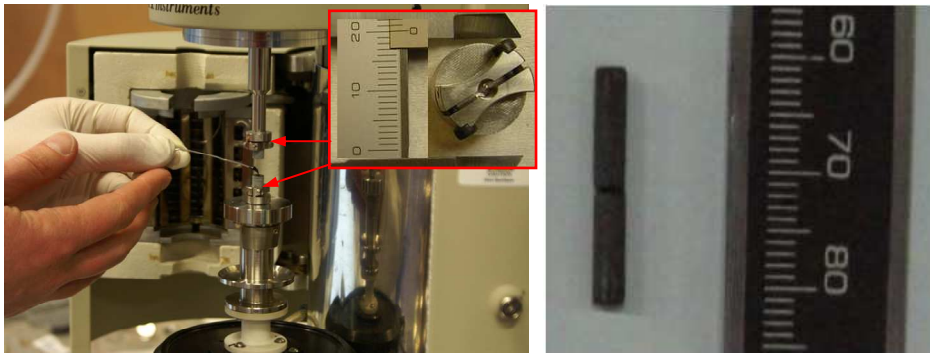
Figure 4.2 Specimen preparation by means of DSR (left) and the overview of the specimen that is used for DMA uniaxial tensile testing (right)
