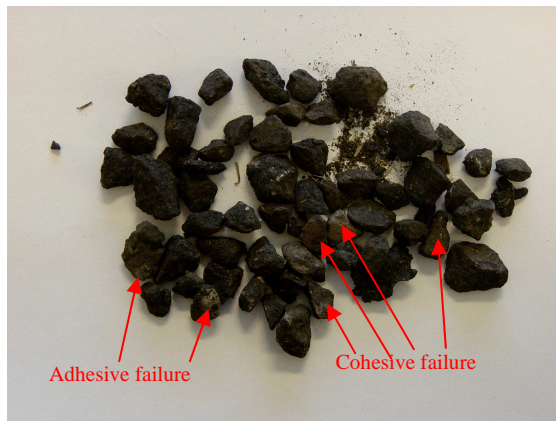
Figure 1.3 Ravelled coarse aggregates indicate the type of failure
