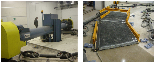
Figure 8.3 Overview of APT at STUVA (left) and some parallelograms that combined make the test section (right)
