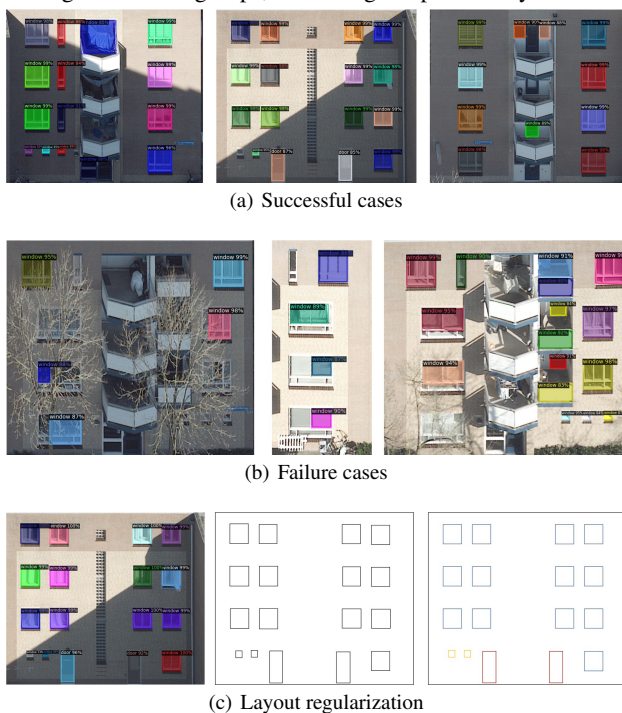
Figure 10. Mask R-CNN façade opening detection results.
