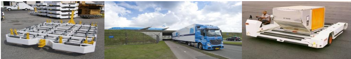
Figure 12 from the left to the right: Dolly, mega-trailer truck and a pallet mover (de Wit, 2015)
