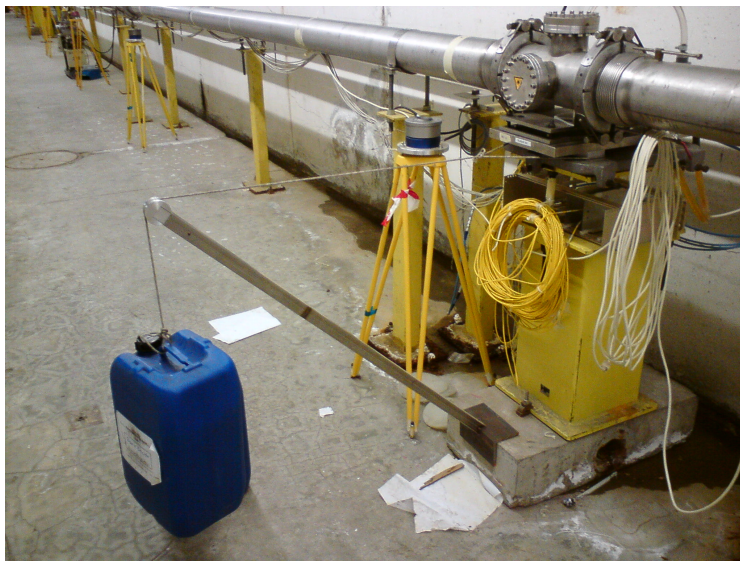
Figure 6.2: Translation applied to the plaque the diffraction plate is on by means of a pulley and a weight (tank filled with water). Two WPS systems (W2D-7D7-006 and W2D-7D7-007) are positioned on the same plaque
