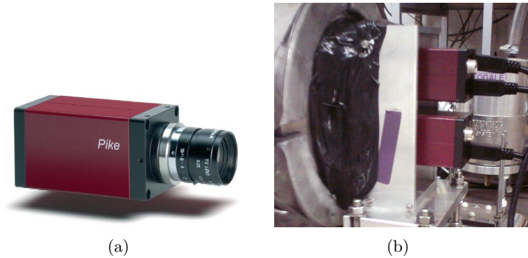
Figure B.9: (a) Catalogue picture of a PIKE100B and (b) two PIKE F100B cams in the TT1 set-up
