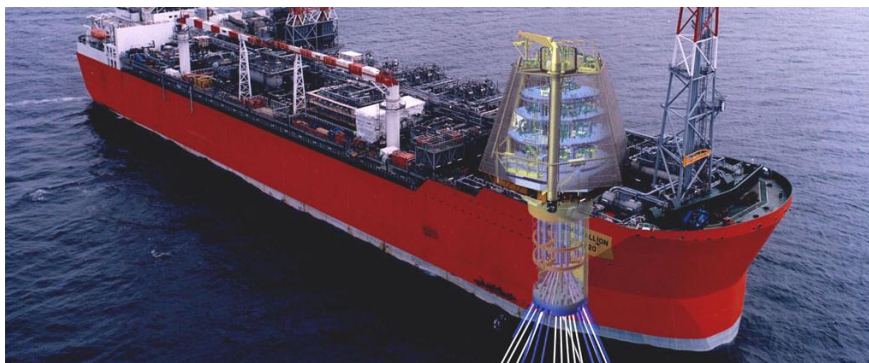
Figure 67 Picture of a Turrets Mooring System
