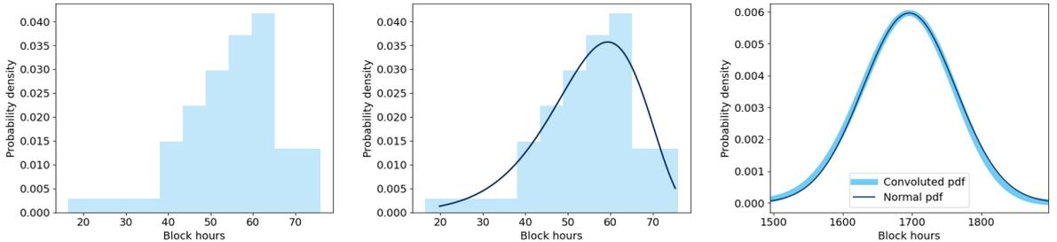
(a) Original histogram of the data. (b) Beta probability distribution fit- (c) Convoluted Beta distributions and theoretical normal distribution.
