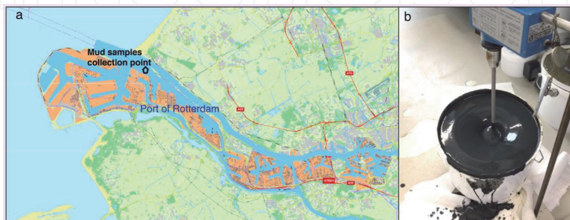
Figure 1. (a) Map of the port of Rotterdam illustrating the location of the site from where the fluid-mud samples had been collected (source: Google maps). (b) The process of homogenizing fluid mud with a mechanical mixer.
