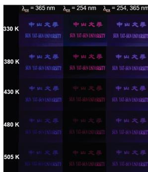
Fig. 7 Luminescent images of patterns formed by  $\text{Ca}_{0.98}\text{Eu}_{0.02}\text{MgSi}_2\text{O}_6$  sample synthesized under  $\text{N}_2$  ambience with different excitation wavelength and temperature.
