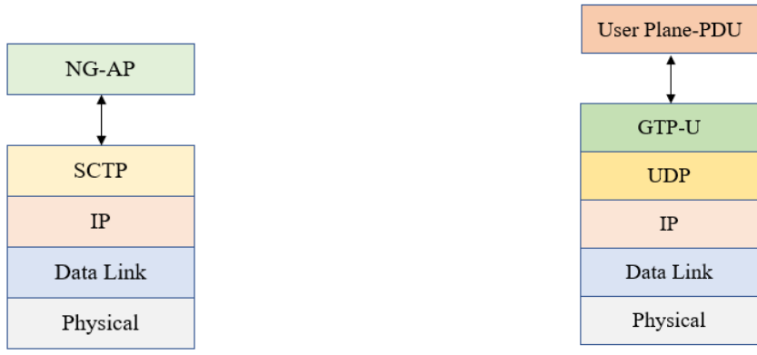
(a) gNodeB and Core network control plane (b) gNodeB and Core network user plane
