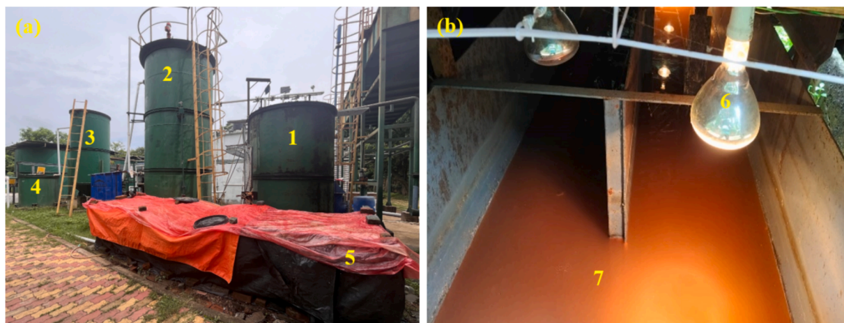
Fig. 1. Set-up of raceway-pond coupled with high-rate anaerobic digester: (a) 1-Feed tank; 2-High-rate anaerobic fermenter; 3-Lamella settler; 4-Neutralisation tank; 5-Raceway pond; (b) 6- Incandescent infrared bulb; 7-Growth of PNSB in raceway pond.
