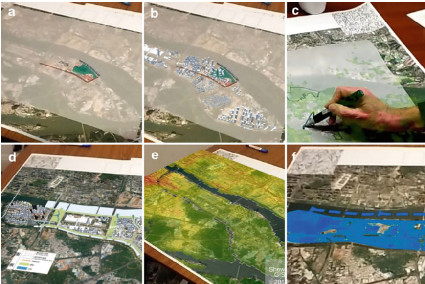
Fig. 9.2 Views of the cartographic AR application: a the base map and tracing paper; b augmented 3D buildings onto the designs; c a participant annotating the map during augmentation; d overlaying 3D models and 2D designs onto the base map; e overlaying GIS data; f overlaying an interactive flood simulation. Photos Adam Tomkins and Eckart Lange
