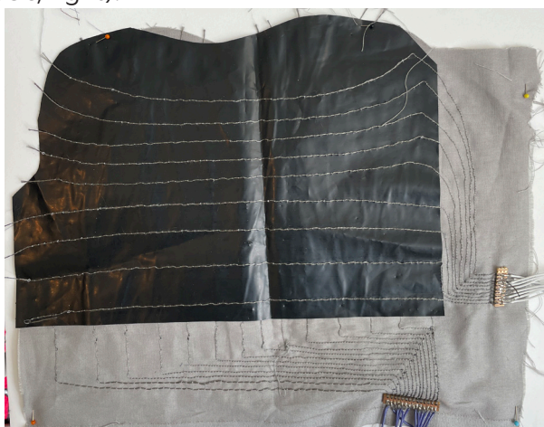
Figure 40. Ambitious large matrix constructed with faulty wire connections
