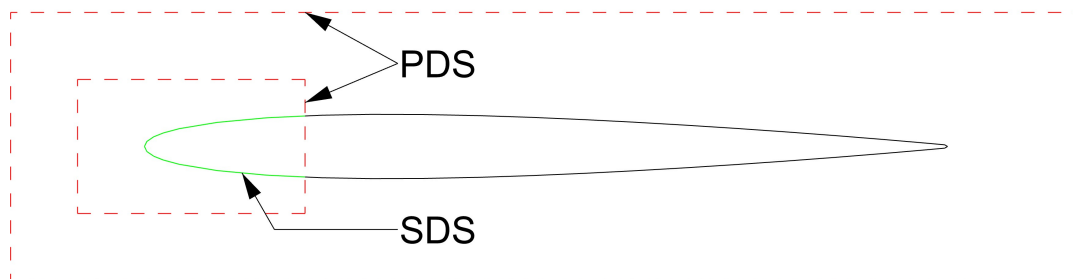
Figure 3.5: Examples of choices for the porous data surface (PDS) and solid data surface (SDS) for the FW-H analysis.
