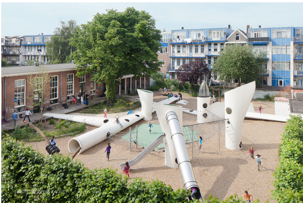
Figure 3. The playground Wikado after the application of the new external layer of coating and paint in 2012. Most of the components of the playground are reused rotor blades, such as the four towers, and the six parts lying horizontally. (Photo by Denis Guzzo, 2014).
