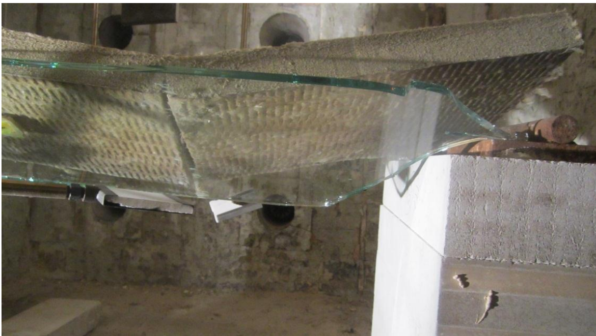
Figure 5.80 Right side pane K after break
