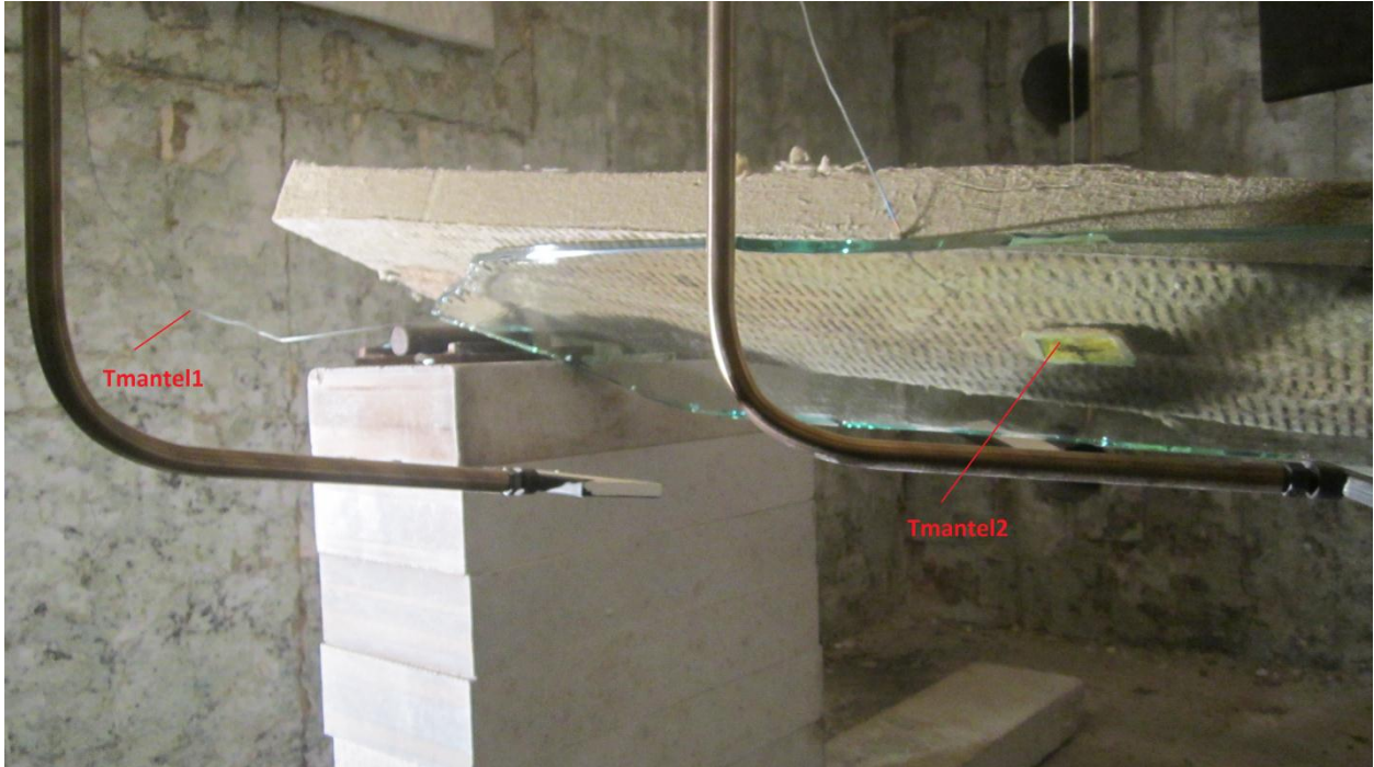
Figure 5.82 Used mantelcouples for temperature measuring
