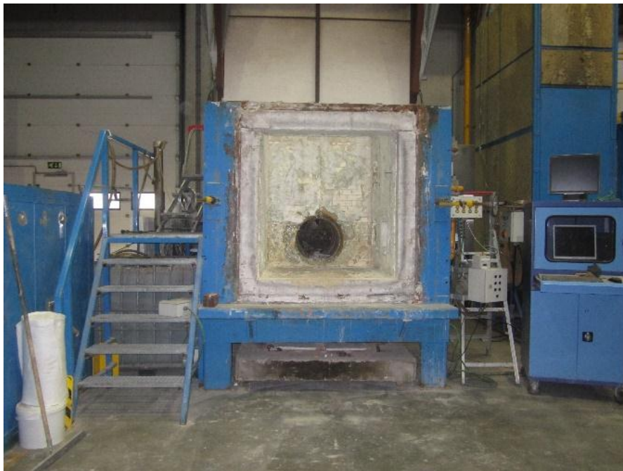
Figure 5.8 Front side small furnace
