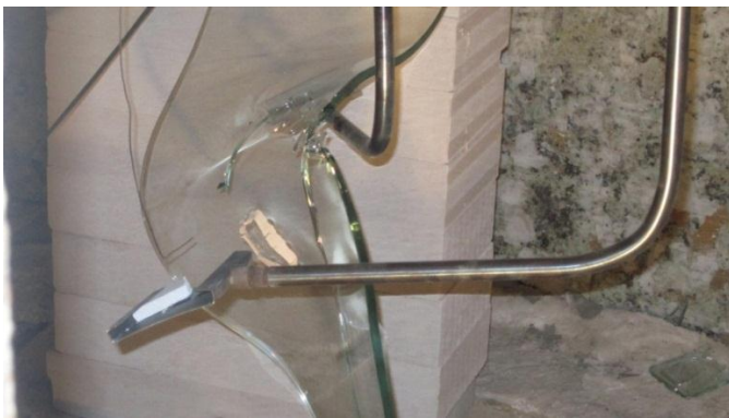
Figure 5.105 Thermal break pane N
