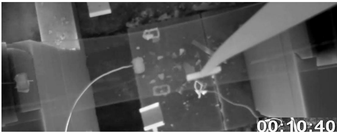
Figure 5.126 Pane M before fail after 10:40 minutes
