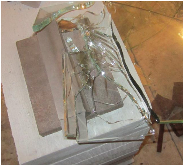
Figure 5.108 Used promatect isolation after test
