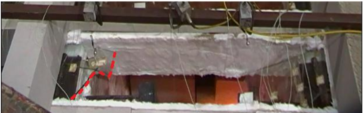
Figure 5.29 pane A after break
