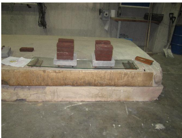
Figure 5.42 Glass pane with 84 kg vertical load at room temperature
