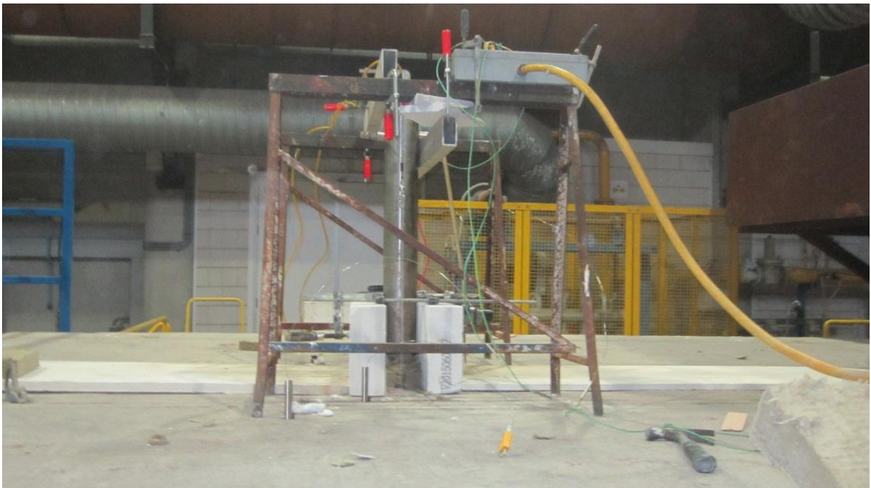
Figure 5.70 Oven camera and deflection measurer
