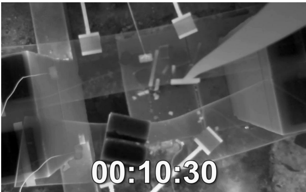
Figure 5.99 Pane O behavior after 10.30 minutes
