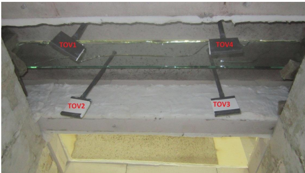
Figure 5.55 Bottom glass pane D view with location of installed plates thermometers
