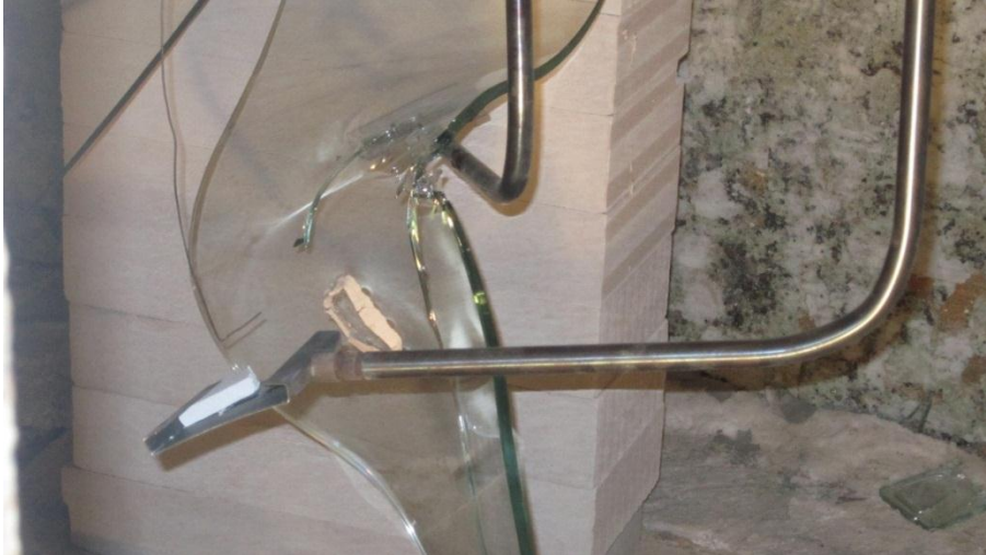
Figure 5.94 Thermal break after testing pane N
