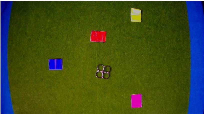
Figure 6.6: Overhead view of Cyber Zoo with quadrotor and color-based vision features
