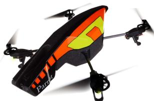
Figure 2.5: The AR.drone 2.0 is a relatively inexpensive quadrotor MAV that can be purchased for recreational uses or for research. Picture credits by Parrot.com
