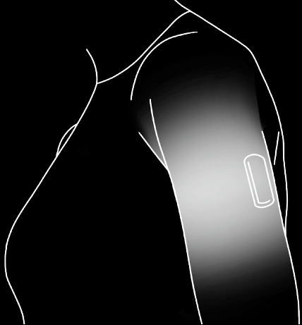
Sewing the shirt tighter to secure stability of the upper arm IMU
