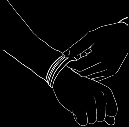
Anti-slip elastic at wrist to secure stability of the lower arm IMU
