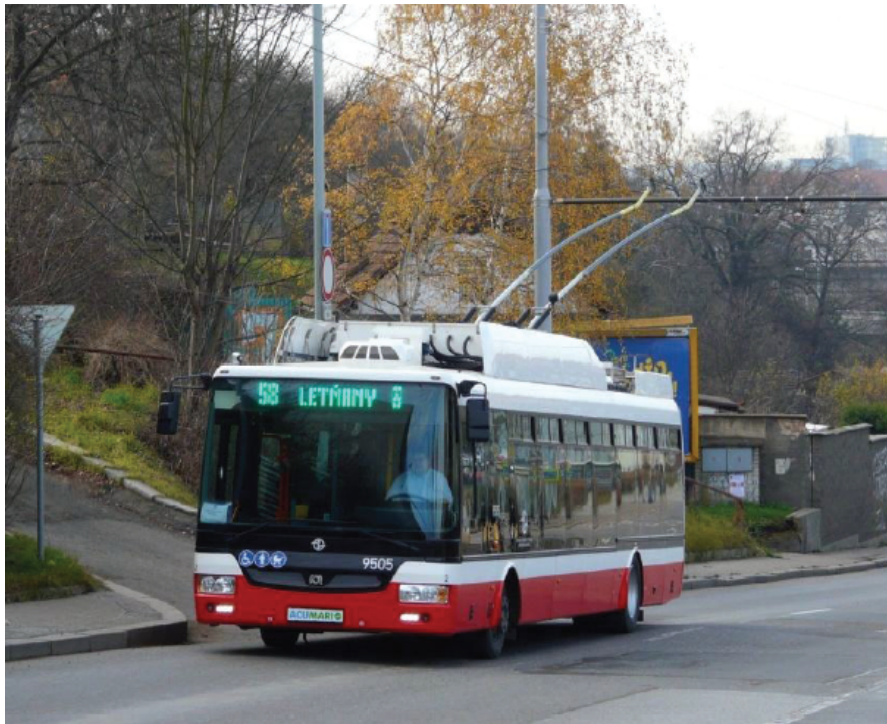
Figure 1.1: Trolleybus connected to a trolley-grid via current collectors [2]
