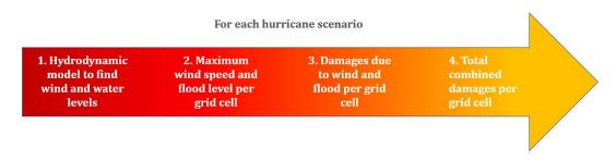
Figure 3.25: Flow chart of how to determine damages per hurricane.
