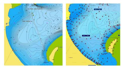
Figure 3.5: Left: Sonar details of depth contours for Orient Bay, St. Martin (Navionics, 2019). Right: Geo-referenced image with point data along different depth contours to extract depth data along the shore.
