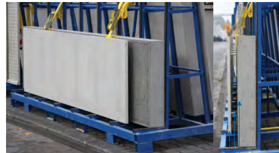
Sandwich panel with a UHPC face wythe UHPC face wythe GFRP connector support structure
