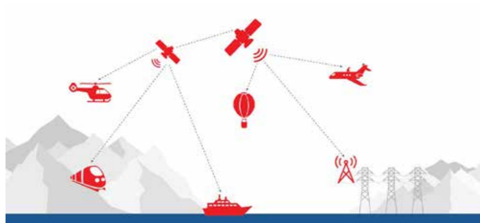
image / figure 2: In NTN's individual objects communicate directly with the satellites
