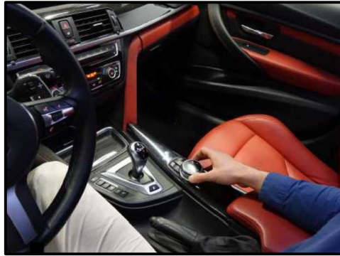
Figure 2.5: A rotary rating knob to extract rating values. Adapted from Ellensohn et al. [2019].
