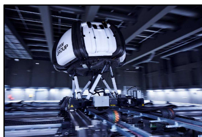
(f) Sapphire Space (xy-drive, hexapod, yaw-drive).
