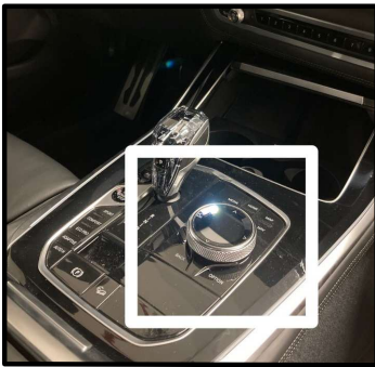
(c) The iDrive rating knob, used for the extraction of the continuous Motion Illness Symptoms Classification (MISC) values.
