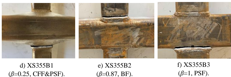
Fig. 6.7 Failure modes of S355 X-joints.
