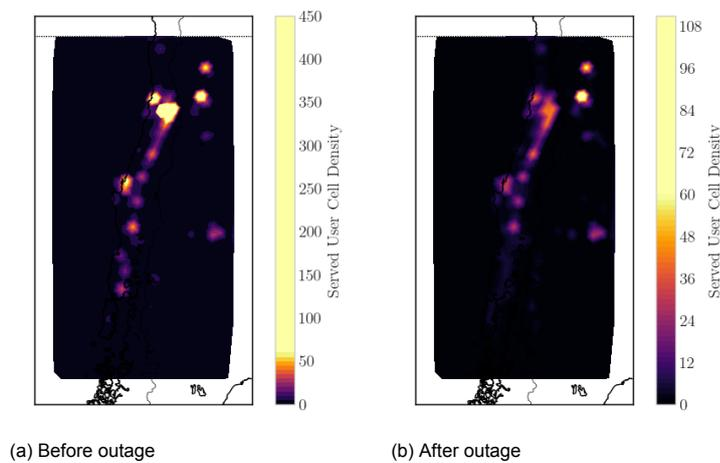
Figure B.1: The effect of the Chile earthquake on the regional capacity for OneWeb
