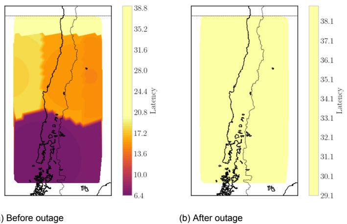
Figure B.7: The effect of the Chile earthquake on the regional capacity for Amazon LEO Initial
