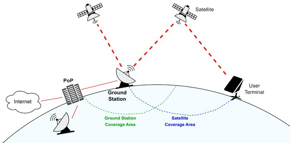
Figure 2.1: Overview of the main components in a satellite internet network
