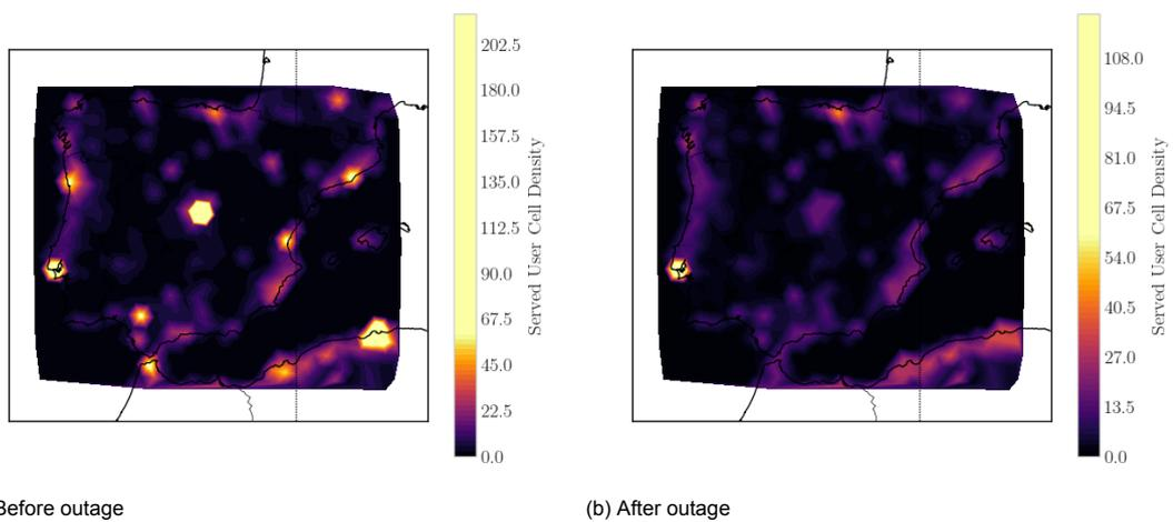
Figure B.10: The effect of the Iberian blackout on the regional capacity for OneWeb
