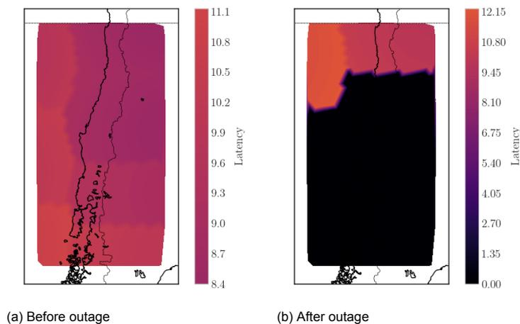
Figure 5.7: The regional propagation latency of OneWeb during the Chile earthquake scenario. Black areas indicate regions with no coverage.
