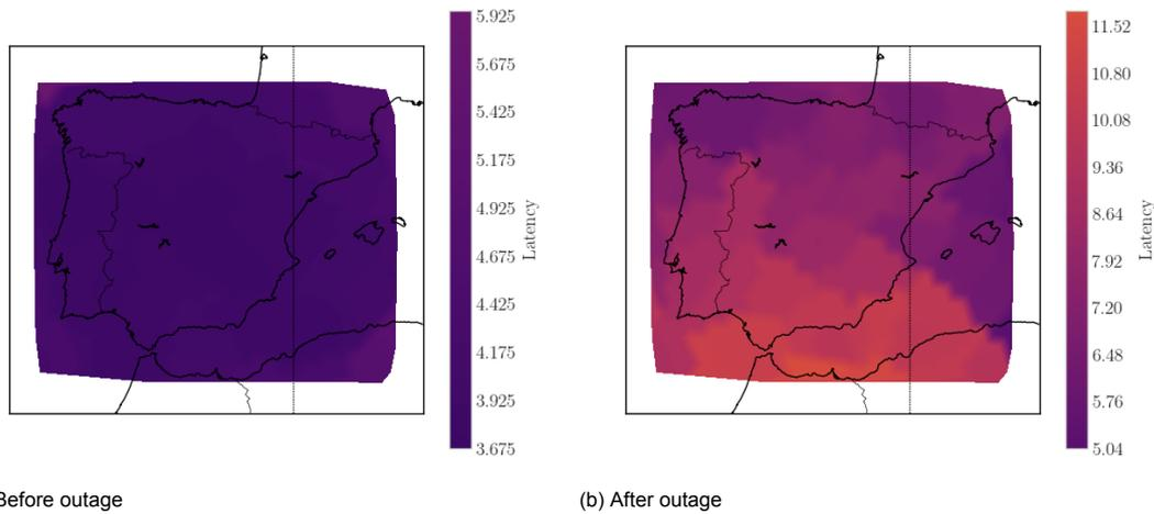
Figure 5.8: The effect of the Iberian blackout on the regional latency for Starlink
