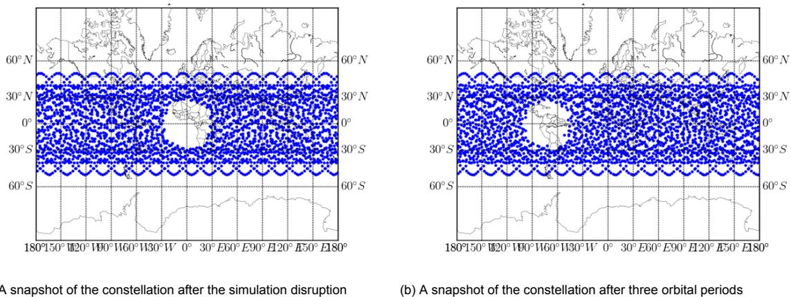
Figure 5.15: Propagation of a satellite cluster over time for Amazon LEO (generation 1)
