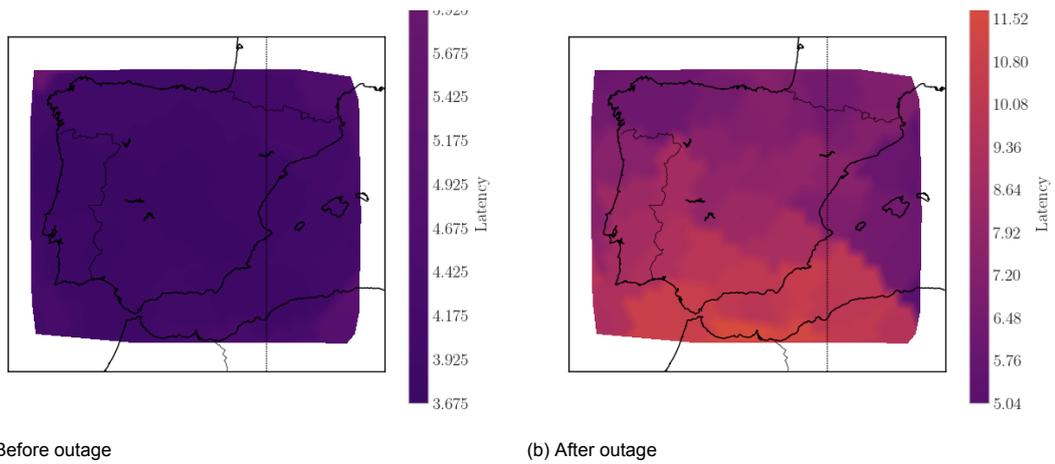
Figure B.14: The effect of the Iberian blackout on the regional capacity for Starlink
