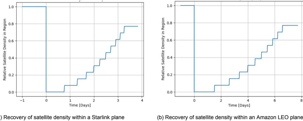
Figure 5.14: Estimated recovery of satellite density
