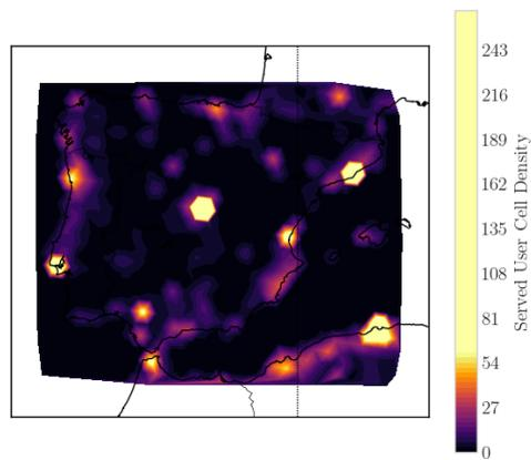
Figure B.13: The regional capacity for the full Amazon LEO constellation. This remains identical after the disruption.
