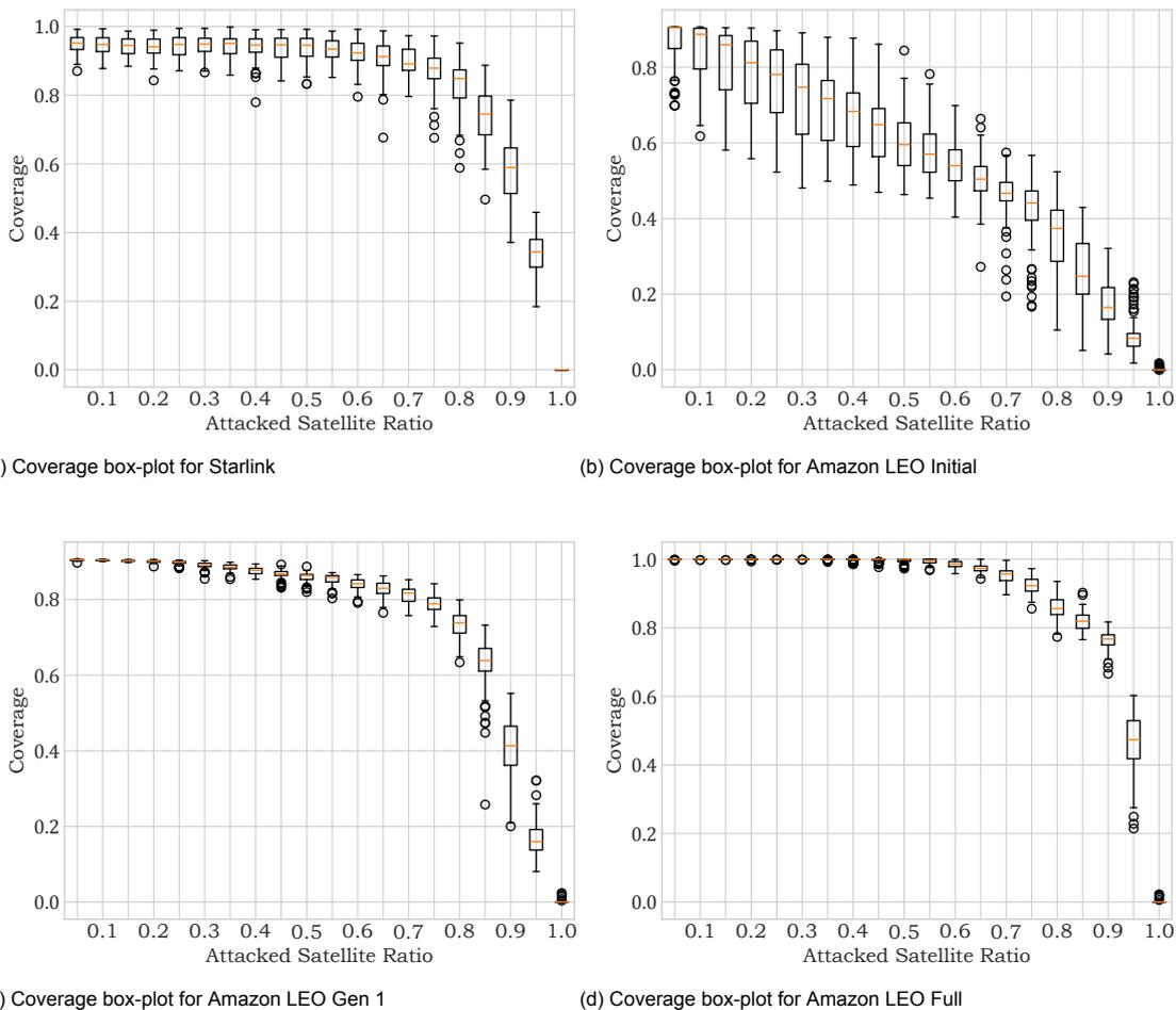
Figure 5.2: Box-plots of satellite coverage vs attack ratio for Starlink and Amazon LEO
