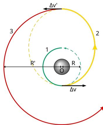
Figure 2.3: Illustrative example of a transfer orbit [34].
