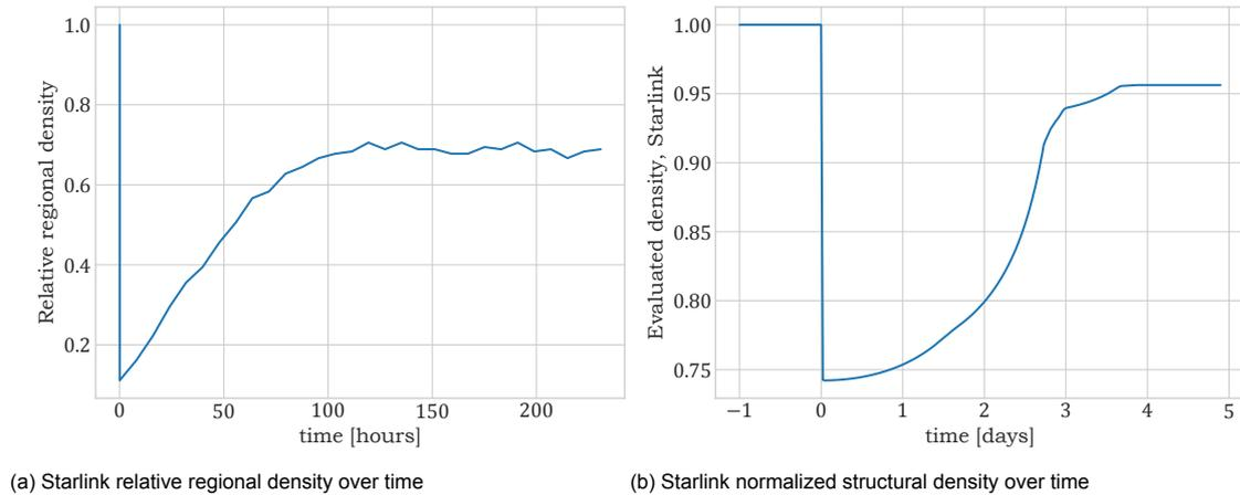
Figure 5.16: Density recovery of Starlink satellites
