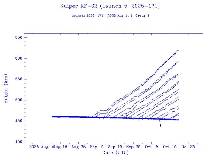
Figure 5.11: Orbit-raising of an Amazon LEO satellites from the KF-2 launch in 2025 [40].
