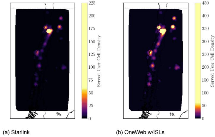
Figure B.2: The regional capacity in Chile for Starlink and OneWeb w/ISLs, these remain identical after the disruption.
