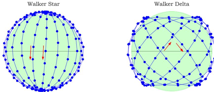
Figure 2.2: Illustrations of basic satellite constellation geometries. The red arrows indicate the direction of motion within the satellite planes.
