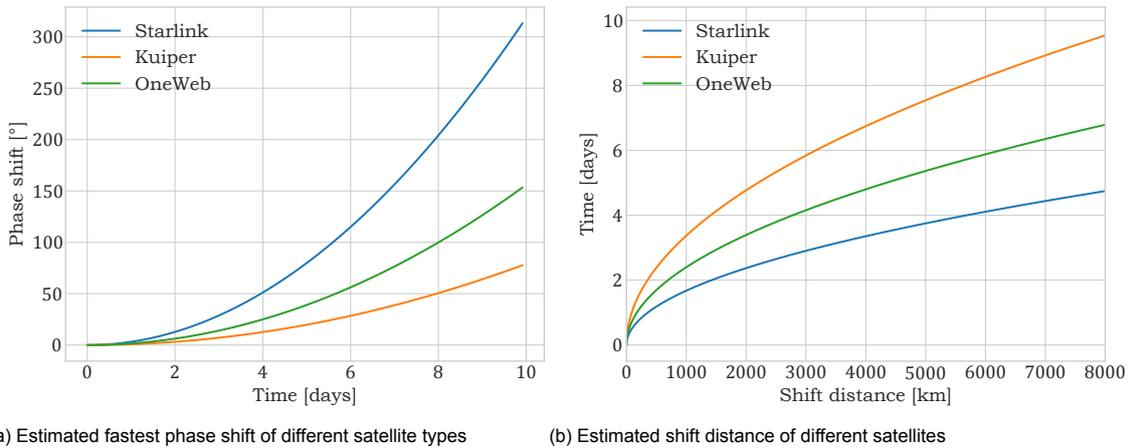
Figure 5.12: Estimated maneuvering capabilities of satellites
