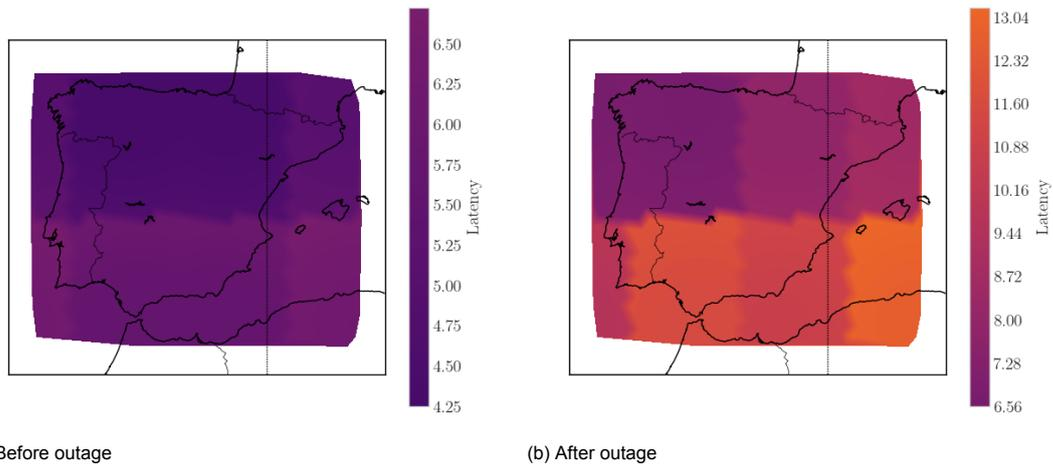
Figure B.17: The effect of the Iberian blackout on the regional capacity for Amazon LEO Initial
