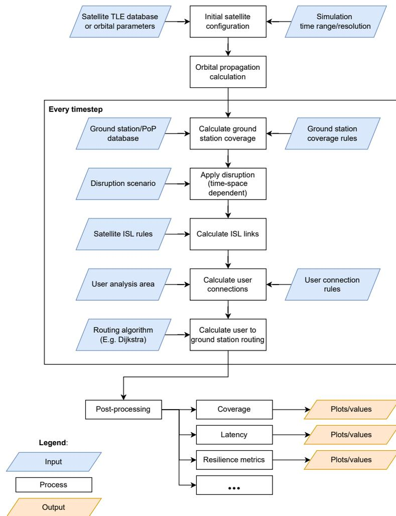
Figure 4.1: Overview of the resilience analysis simulation tool.
