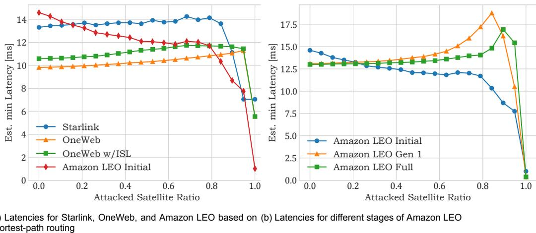
Figure 5.4: Estimated mean propagation latencies vs attack ratio based on shortest-path routing
