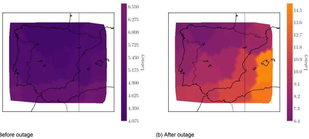
Figure B.18: The effect of the Iberian blackout on the regional capacity for Amazon LEO Generation 1
