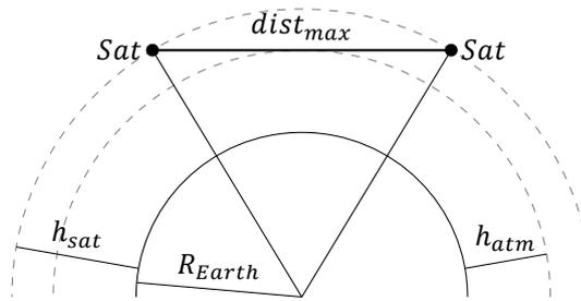
Figure 4.3: Illustration of the physical ISL distance limit
