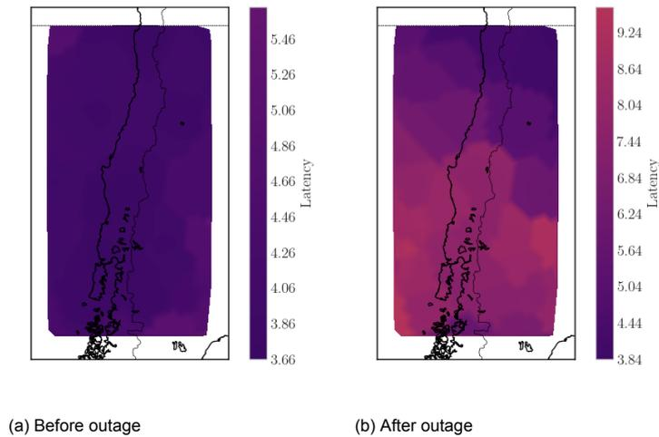
Figure 5.6: The regional propagation latency of Starlink during the Chile earthquake scenario
