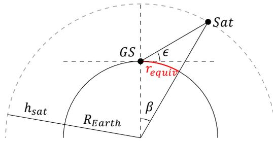
Figure 4.2: Illustration of the coverage area
