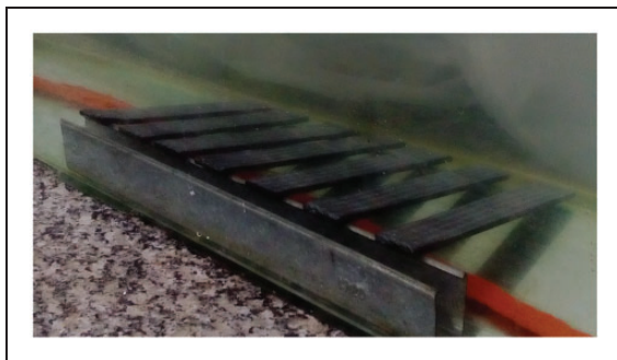
Figure 2. Specimens inside the salt water tank.
