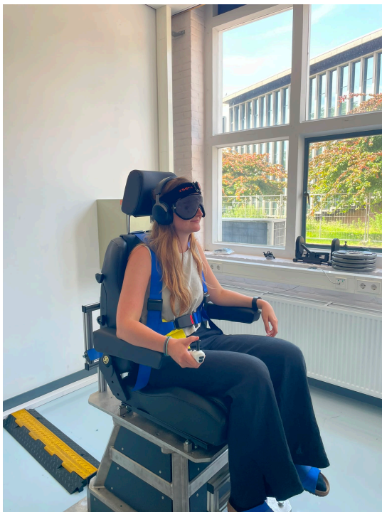
Figure A.1: Participant set-up for the rotational motion perception test, including a blindfold, noise-canceling headphones, a handheld response lever, and an IMU sensor placed on the head
