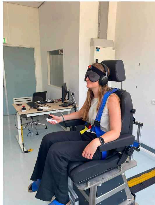
Figure A.1: Participant set-up for the rotational motion perception test, including a blindfold, noise-canceling headphones, a handheld response lever, and an IMU sensor placed on the head
