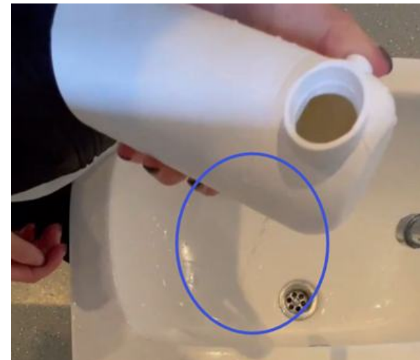
Fig 5.3.4 Observed water leak when horizontally hold the canister
