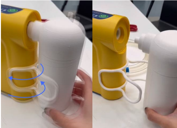
Fig 5.3.5 Image made by superimposing video screenshots (left) disconnecting the canister (right)
