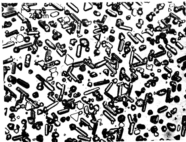
Fig. 5. Optical micrograph. Mean thickness: about 1 \mu\text{m} ; current density: about 1.5 \text{mA}/\text{cm}^2 .
