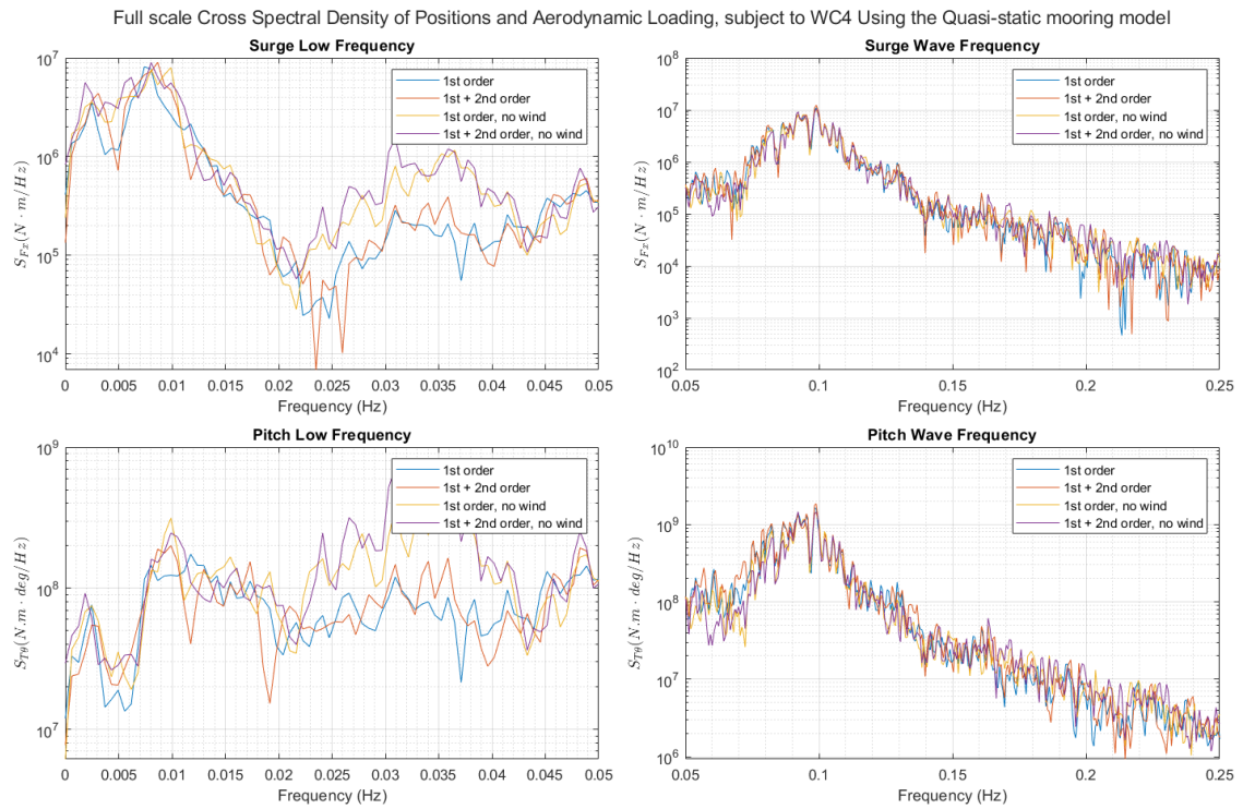
Figure D.4: Cross Spectral Density of aerodynamic surge force & surge position, and Aerodynamic pitching moment & pitch inclination, subjected to WC4.
