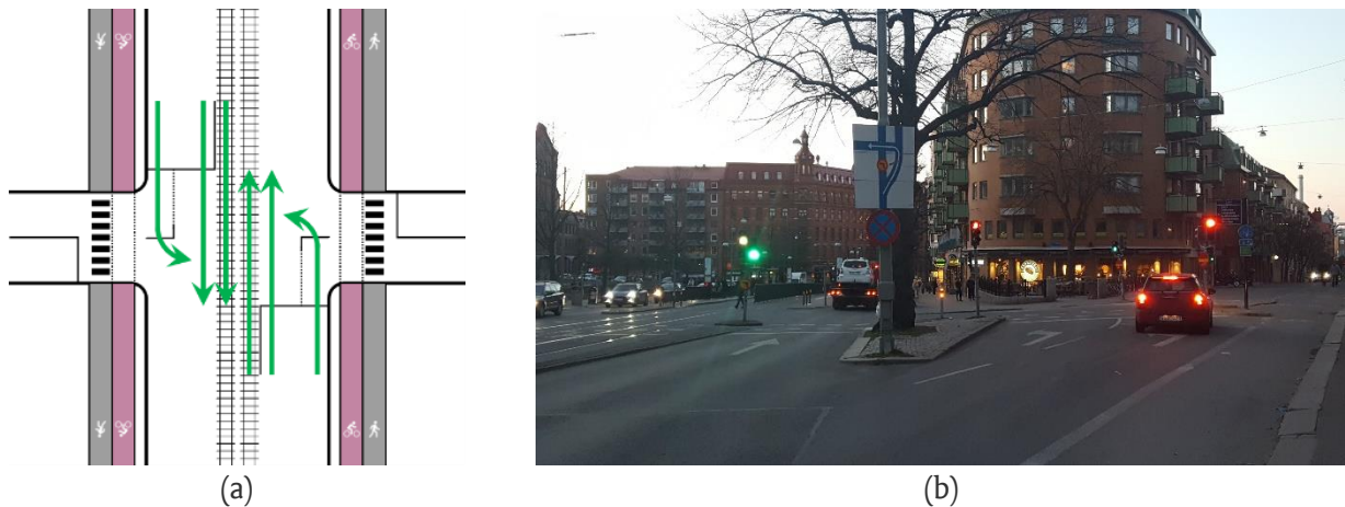
Figure 2-6 | Illustrations of permitted conflict type 5 (hook turns) in a right-driving system, with (a) a schematic overview, and (b) implementation in practice in Gothenburg, Sweden.
