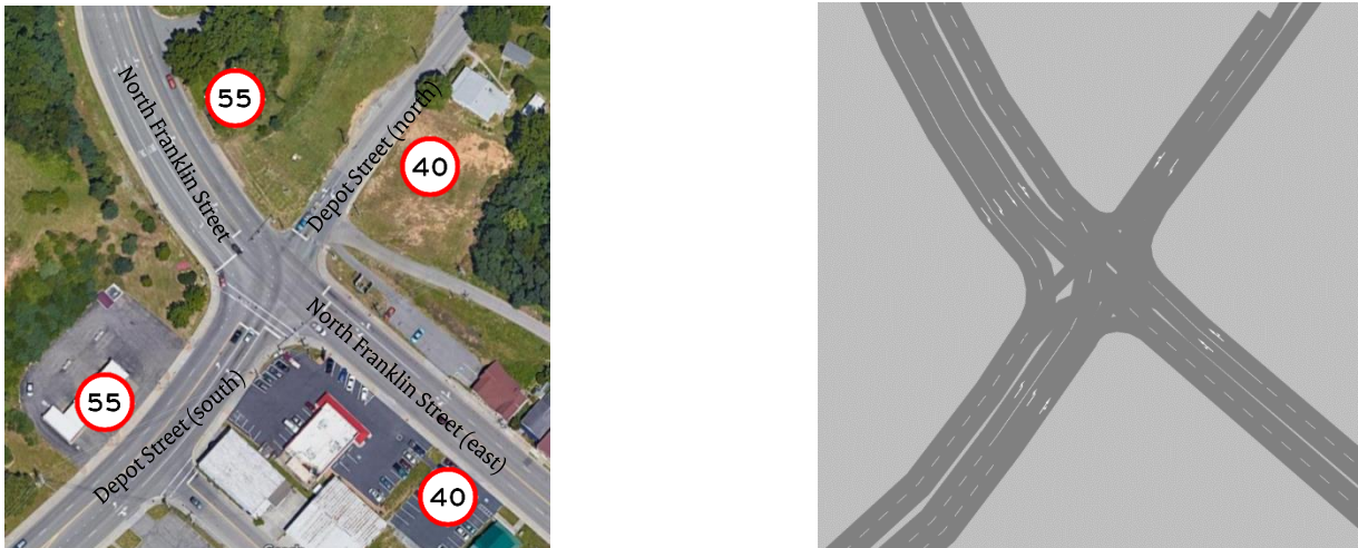
Figure 5-1 | Satellite image (left; Google Maps, 2018), and corresponding VISSIM model (right) of the signalised intersection in Christiansburg, Virginia, U.S.A., with maximum speeds in kilometres per hour (Zohdy, Sadek, & Rakha, 2010).
