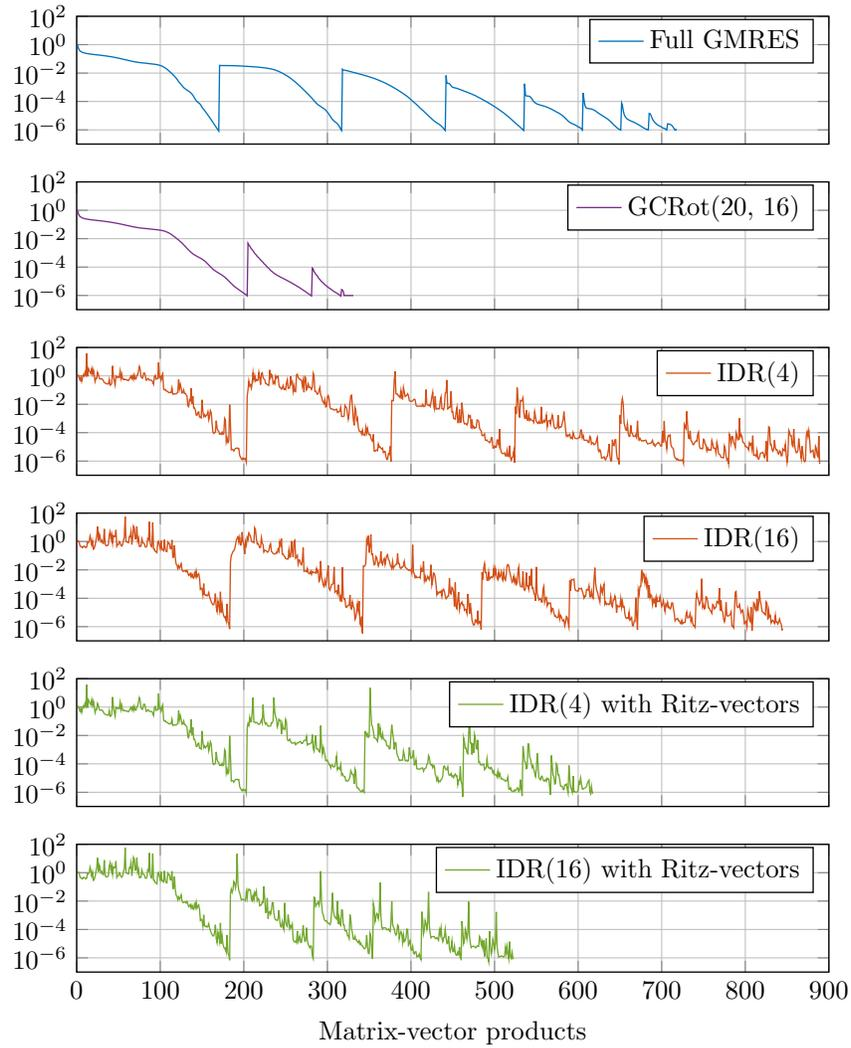
Figure 7: (*Example 7*). Convergence residual history for the solution of (32) (diffusion-dominated example)
