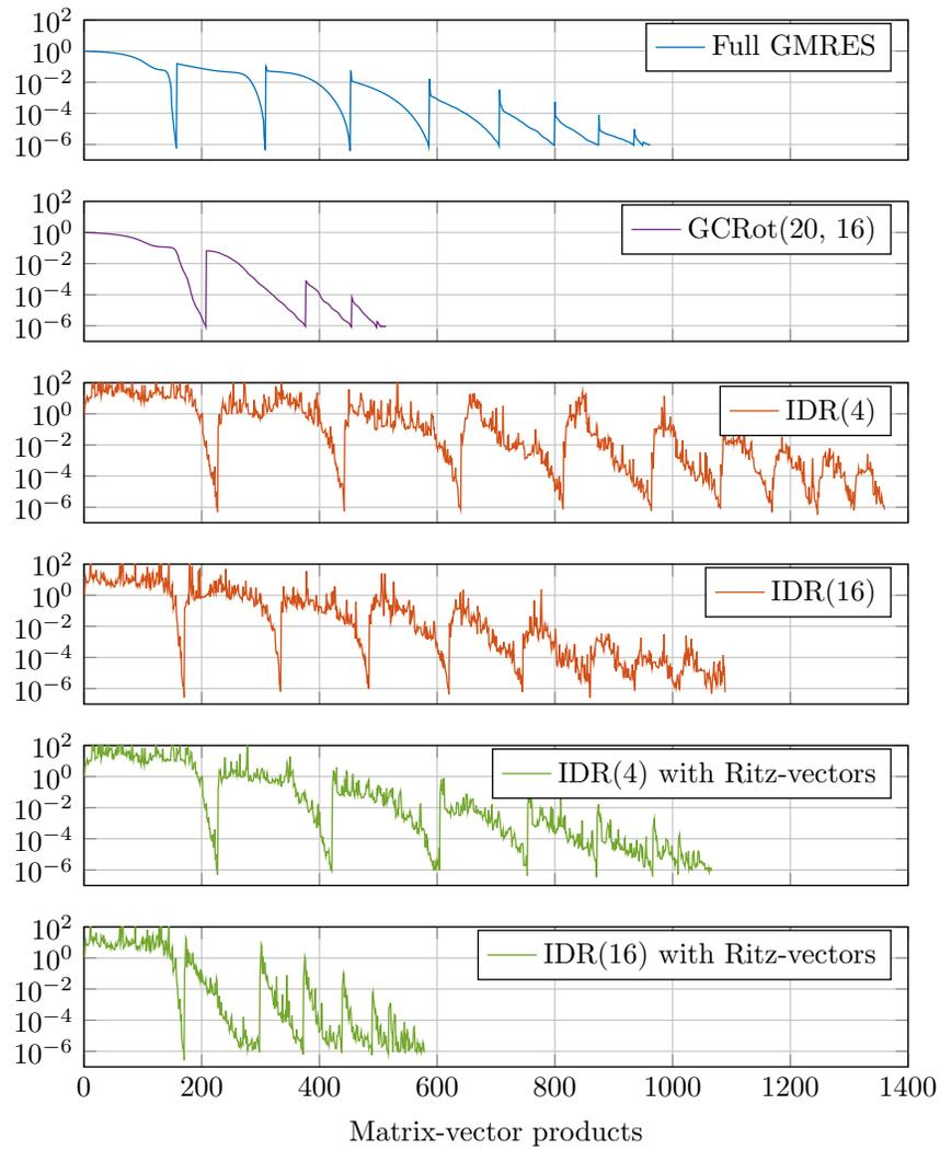
Figure 8: (*Example 7*). Convergence residual history for the solution of (32) (convection-dominated example)
