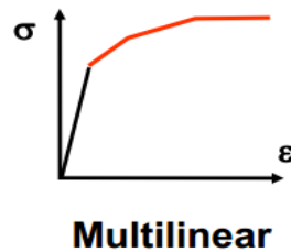
Figure 3.3: Multilinear isotropic hardening material input in ANSYS
