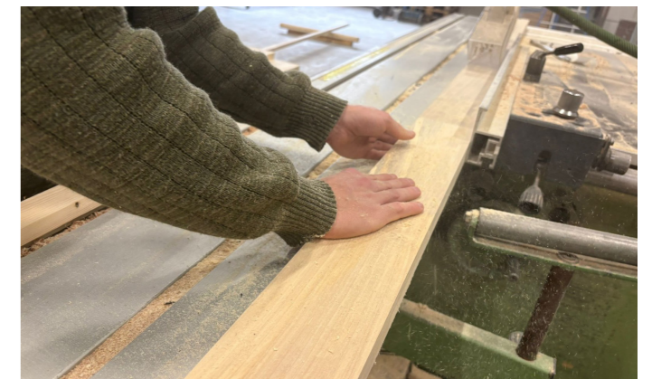
Figure 26: Planing fingerjointed and laminated poplar beams
