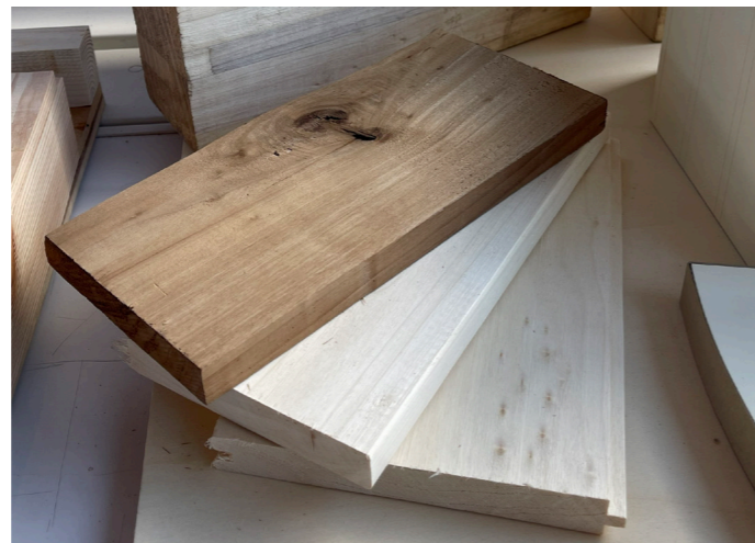
Thermally modified poplar and unmodified poplar for interior and exterior finish
