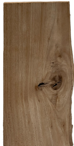
Thermally modified poplar timber after lying outside for three weeks
