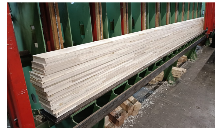
Figure 25: Fingerjointed and laminated poplar beams
