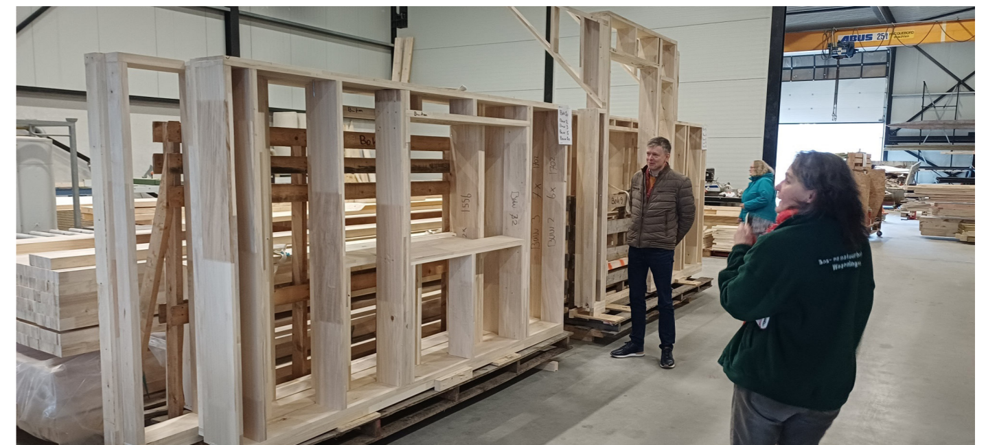
Figure 33: Prefabricated poplar timber frame elements
