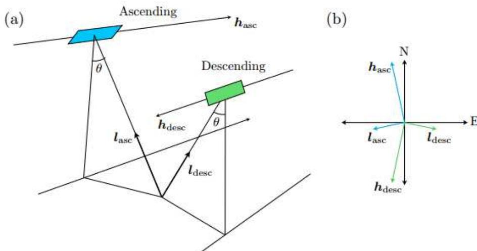
Figure 2.10, (a) Geometry for ascending and descending satellite directions. (b) Projection of heading and LOS vectors onto the ground, with "l" as LOS and "h" as heading. (Wortham, 2014)
