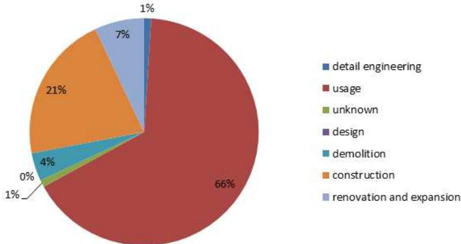
Figure 3.2, Phase in which failure is discovered. Source: Terwel (2012), *Constructieve incidenten in Cobouw 1993-2009*
