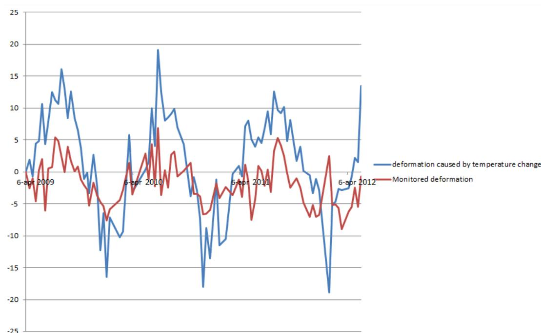
Figure 5.20, Graph of the relative temperature and the displacement per measurement. In red the monitored displacement and in blue the calculated movement by temperature difference. The data is provided by Hansje Brinker. The data of the satellite is recorded with the TerraSAR-x satellite. The temperature is from the KNMI.
