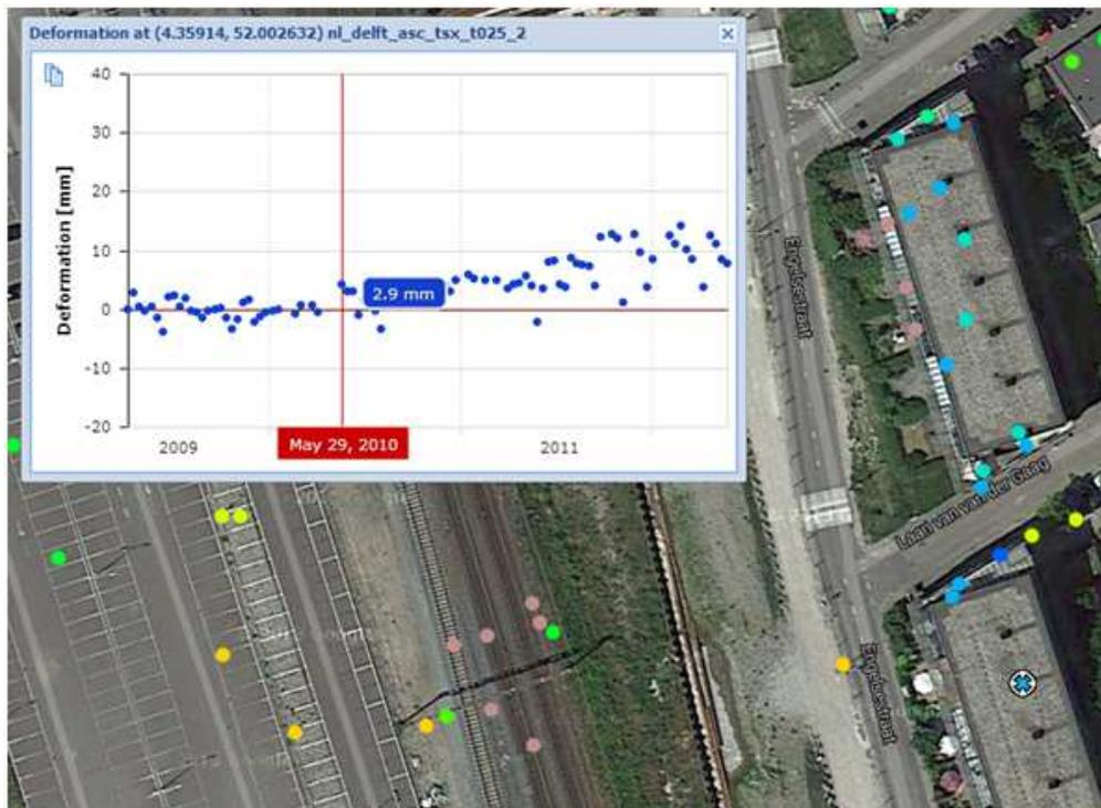
Figure 5.8, deformation of the white marked satellite point started to rise at the end of May. The data is provided by Hansje Brinker. The data of Delft is recorded with the TerraSAR-x satellite and projected on Google Maps. The original scale is approximately 1:666.
