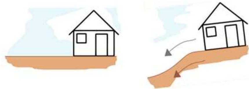
Figure 5.6, a representation of the tilting of the building caused by the subsidence of the soil, caused by the tunnel.
