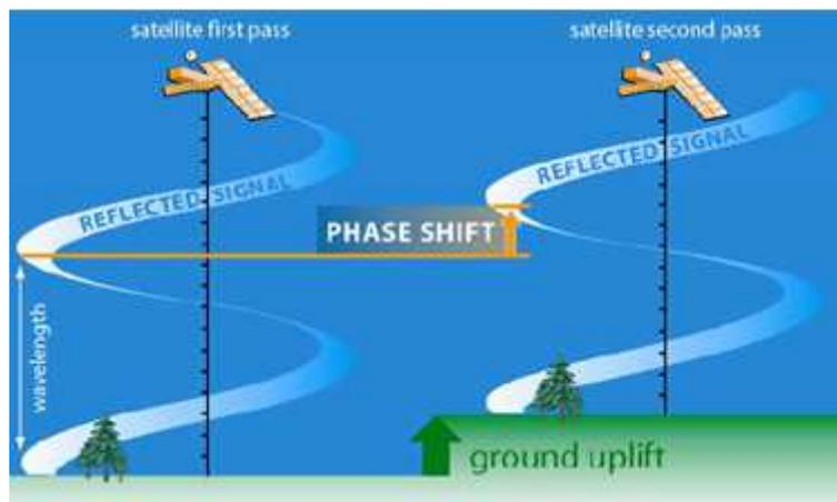
Figure 2.1, An example of the phase difference caused by a displacement on Earth. Source: [www.halliburton.com](http://www.halliburton.com)
