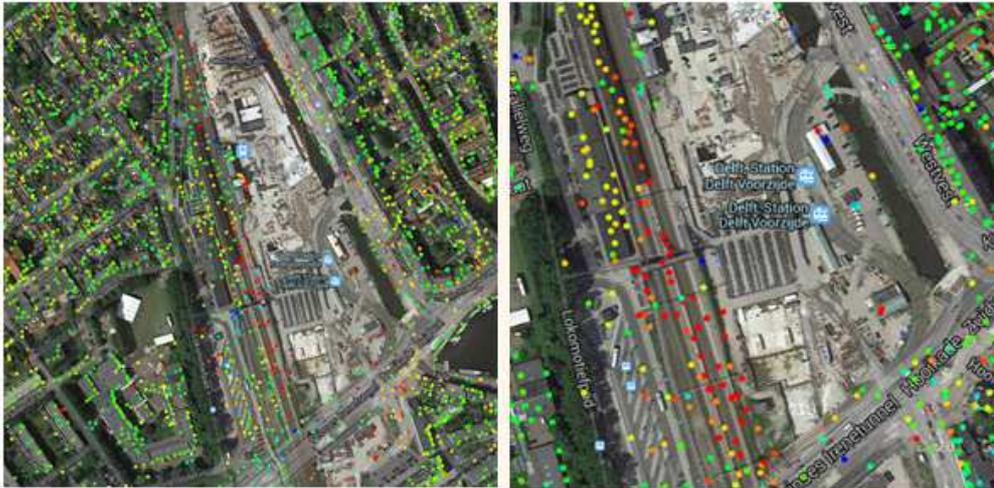
Figure 5.3, in the left figure the descending data of the railway tunnel of Delft. In the right figure the ascending data of the railway tunnel of Delft. The data is provided by Hansje Brinker. The data of Delft is recorded with the TerraSAR-x satellite and projected on Google Maps. The original scale is approximately 1:5000 for the left figure and 1:2500 for the right figure.
