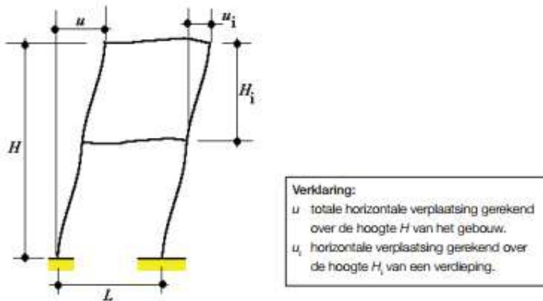
Figure 4.22, Example of horizontal deflection of a framework, according to the Eurocodes. Source: NEN-EN 1990 (2002)
