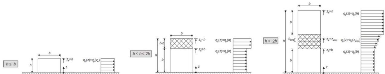
Figure 4.11, Distribution of the wind load to calculate the design wind speed, according to NEN-EN 1991-1-4. (2005)
