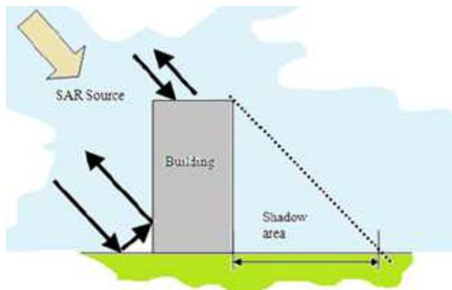
Figure 2.3, Interpretation of a building with a satellite. To the left, arrows reflect double bounce points; in the middle, arrows reflect the building correctly; and to the right, the shadow area caused by the satellite's viewing area can be seen.
