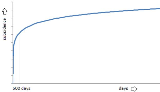
Figure 4.18, Secondary subsidence from 0 days until 10,000 days, so as to demonstrate the equation's characteristics. The subsidence is downwards (in opposite direction of the graph).
