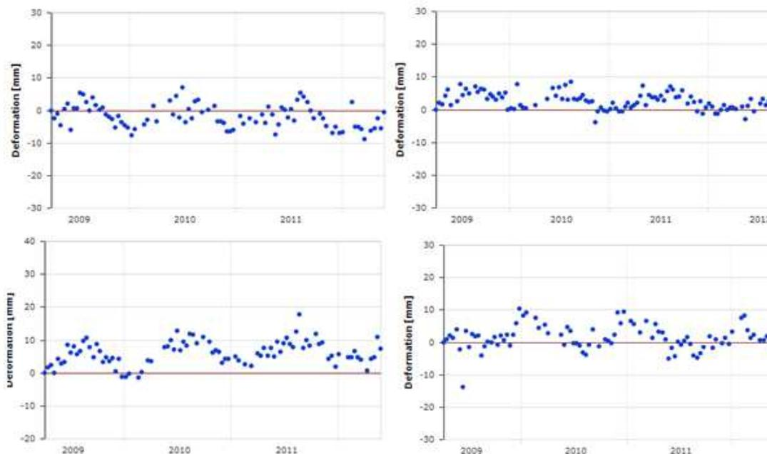
Figure 4.15, Deformation data for Erasmus MC, Delftse Poort, the Millenniumtower, and the World Port Centre from the TerraSAR-x, April 2009 to May 2012.
