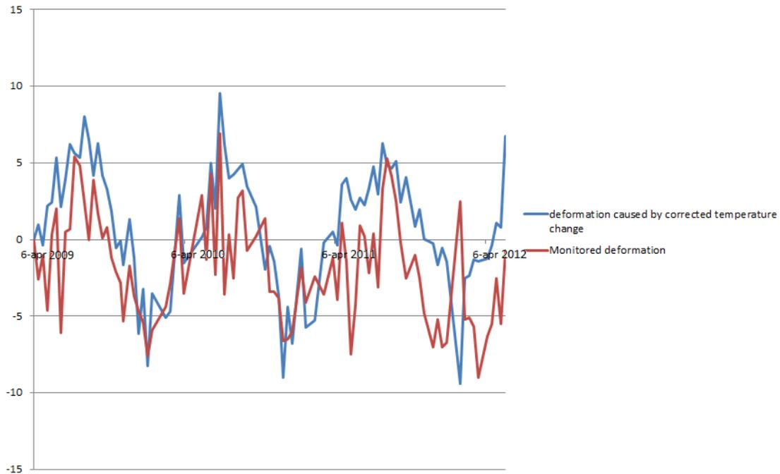
Figure 5.21, calculated corrected temperature deformation is the blue, observed deformation with InSAR in red. The data is provided by Hansje Brinker. The data of the satellite is recorded with the TerraSAR-x satellite. The temperature is from the KNMI.
