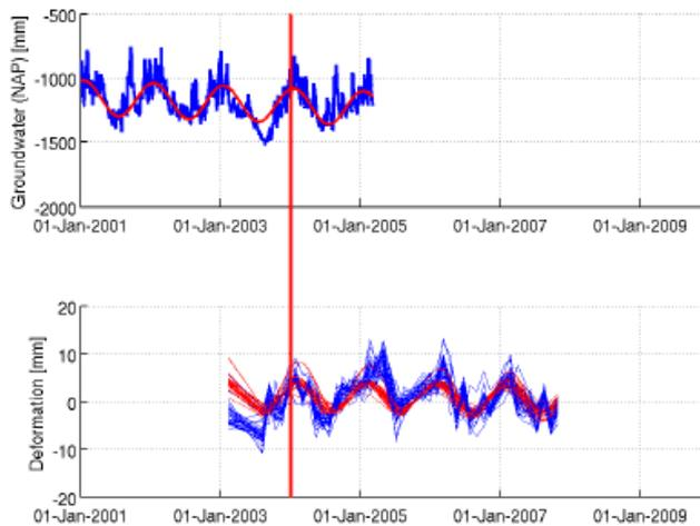
Figure 4.16, The top figure is an example of a groundwater level time series. The other graph shows a PS-point time series. In this figure, indications can be seen that InSAR can monitor the influence of the groundwater on ground deformation. Source: Leijen and Hanssen (2007)
