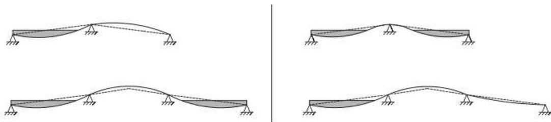
Figure 4.13, Upward and downward movements caused by rain load. Source: NEN-EN 1991-1-3 (2011)
