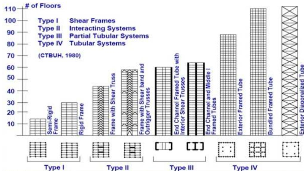
Figure A2.5, stability systems of buildings. Source: Lecture slides of Building structures 2
