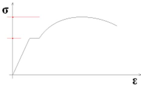
Figure A2.1, A stress-strain diagram of steel. Marked in red is the plastic capacity
