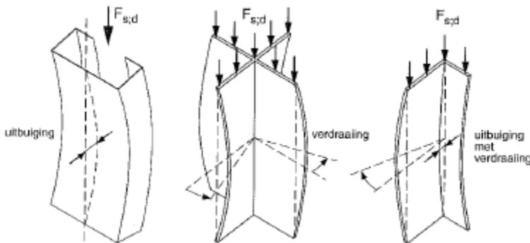
Figure A2.7, beams loaded with compression. Beam left: buckling, middle beam: torsion and right beam: torsional buckling. Source: Reader Construeren A (2001)
