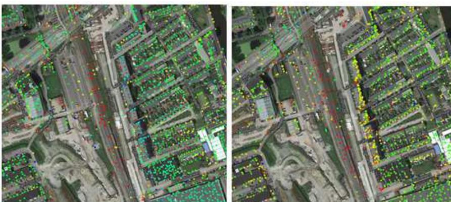
Figures 5.4, the ascending data of houses near the railway tunnel are in the left figure and in the right the descending data of the TerraSAR-x satellite. The data of Delft is recorded with the TerraSAR-x satellite and projected on Google Maps. The original scale is approximately 1:2500.
