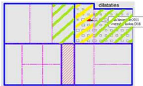
Figure 5.35, the yellow part of the structure is the part where sag can be expected on the roof. The green parts of the structure are the parts where sag can also be expected because of the magnitude in diameter of the sinkhole under the structure.
