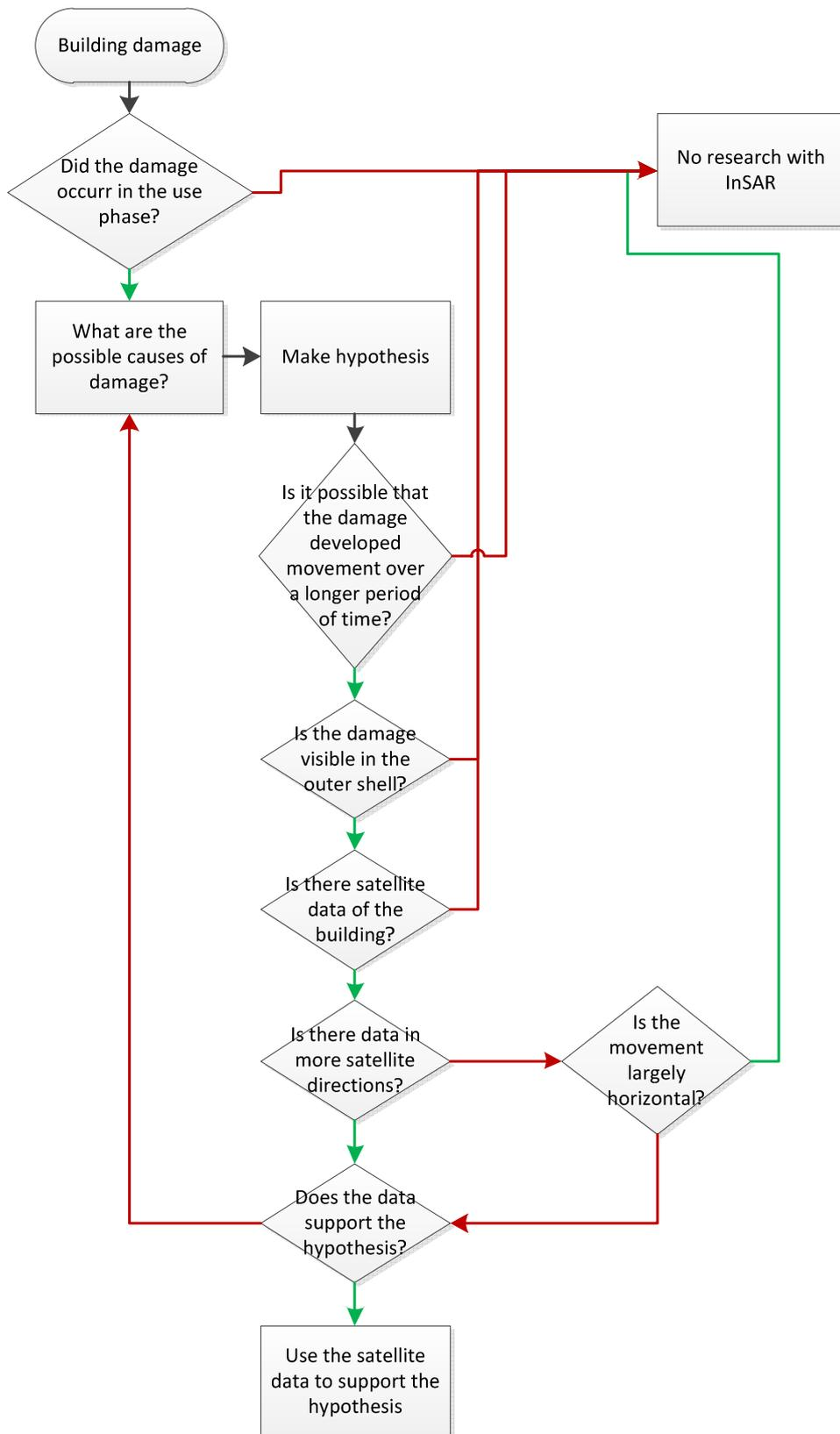
Figure 3.6, The decision tree for using InSAR in forensic engineering to support a hypothesis about a failure mechanism. Diamond shapes are decisions, rectangles are processes, red arrows are negative, and green arrows are positive.
