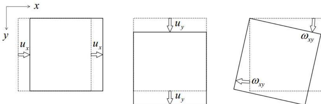
Figure 4.8, Horizontal translation, vertical translation, and rotation, according to elasticity theory. Source: Lecture notes plates and slabs (2011)
