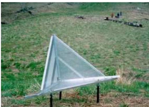
*Figure 4.5, Example of a corner reflector. Source: Central Federal Lands Highway Division (2008)*
