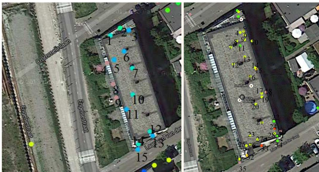
Figure 5.7, the data points of one specific building near the railway tunnel. In the left figure the ascending data and in the right the descending data are seen. The PS-points are numbered for each direction to get a clear overview of the data. The data is provided by Hansje Brinker. The data of Delft is recorded with the TerraSAR-x satellite and projected on Google Maps. The original scale is approximately 1:333.
