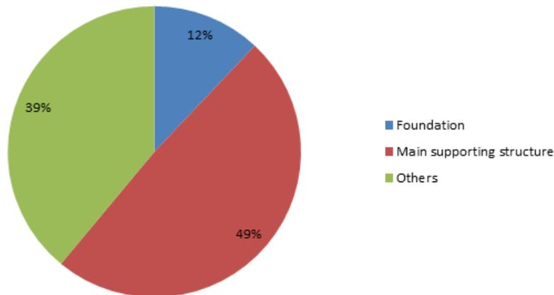
Figure 3.5, Main classification of failed elements. Source: Terwel (2012), *Constructieve incidenten in Cobouw 1993-2009*
