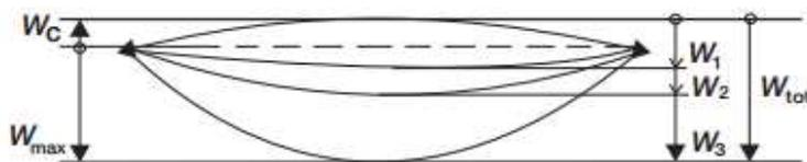
Figure 4.20, Example of vertical deflection of a floor, according to the Eurocodes. Source: NEN-EN 1990 (2002)
