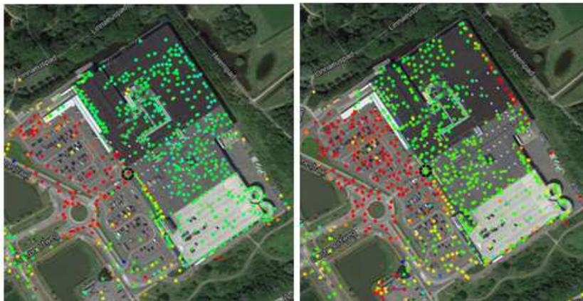
Figure 5.16, ascending data of the Ikea can be seen in the left figure and descending data in the right of the TerraSAR-x satellite. The data is provided by Hansje Brinker. The data of Delft is recorded with the TerraSAR-x satellite and projected on Google Maps. The original scale is approximately 1:6666.
