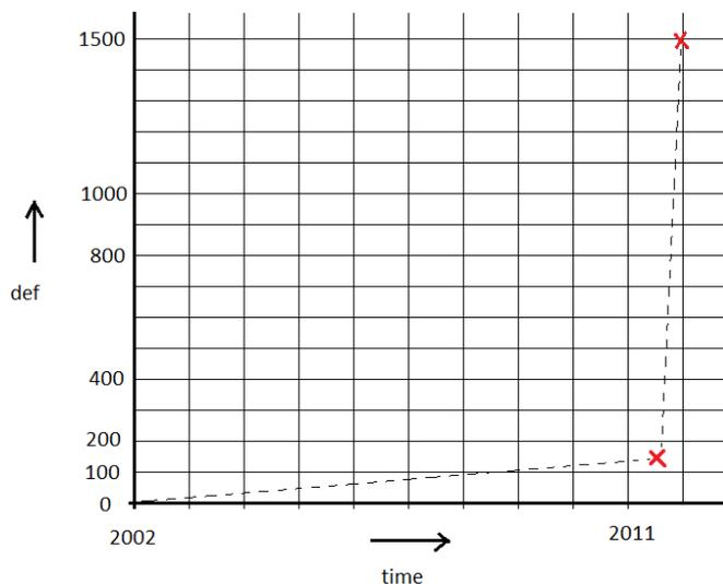
Figure 5.30, graph of certain movement of the column of shopping mall 't Loon at the floor of the parking lot. Deformation is in millimetres.
