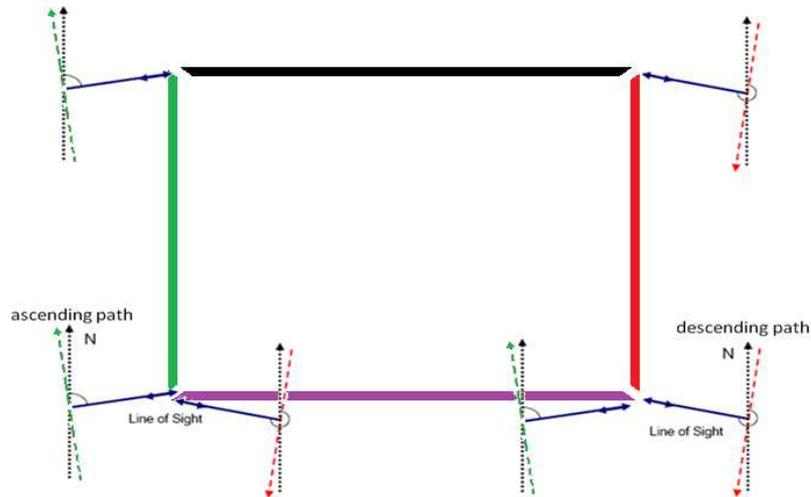
Figure 3.4, A building with façades that match the wind directions. In this case, both the ascending and descending orbit cannot monitor the north façade if the TerraSAR-x satellite is utilized. Green represents the façade that is monitored by the ascending track, red represents the section that is monitored by the descending track, and purple represents the façade that is monitored in both directions.
