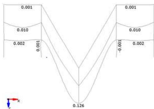
Figure 5.34, sag calculated with MatrixFrame without column 18. The deflection is enlarged to highlight the magnitude of the deflection. Assumed dimensions: (real dimensions unknown) Concrete structure 700x300 mm (columns and first floor), concrete class c25/30. Steel structure I-beam 360x370x134 mm, Steel strength S235. Load on the floors 4 kN/m<sup>2</sup>, on the roof 1 kN/m<sup>2</sup>. A span of 7 metres in both directions is assumed.
