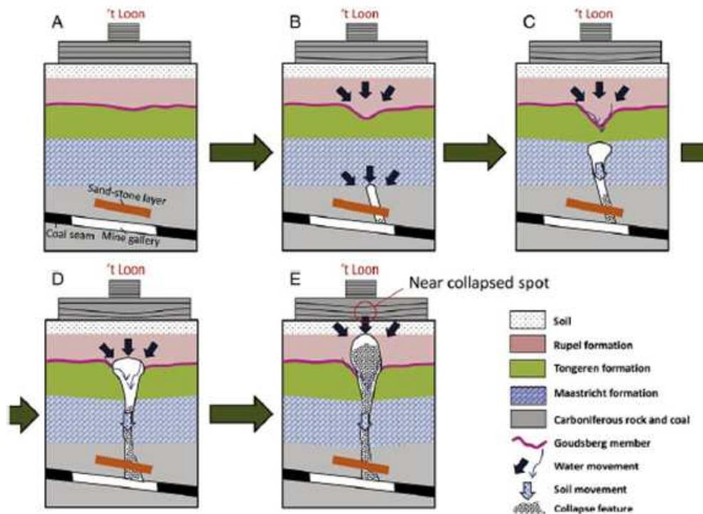
Figure 5.24, developing of the sinkhole in time, source: Detection of cavity migration and sinkhole risk using radar interferometric time series by Chang and Hanssen (2014).
