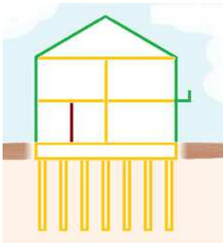
Figure 3.3, Schematization of a building. Green represents the outer shell, yellow the inner supporting structure, and red the non-load-bearing part of the building.
