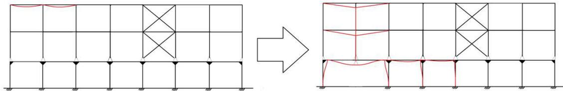
Figure 5.32, theoretical movement of the roof in normal condition and without column 18. The size of the movement is not on scale and is only to give an impression of the movement.
