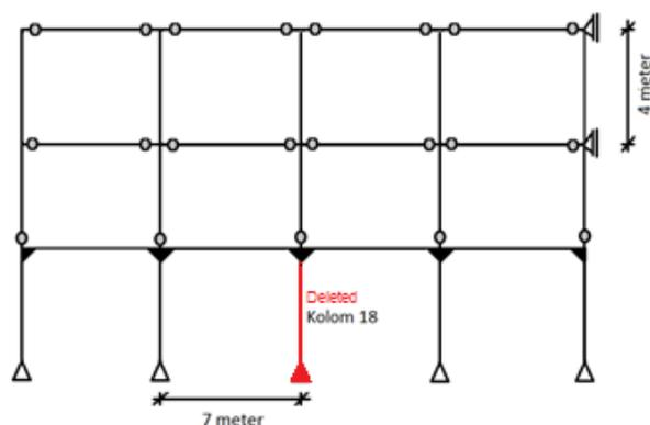
Figure 5.33, starting principles for model in Matrixframe.
