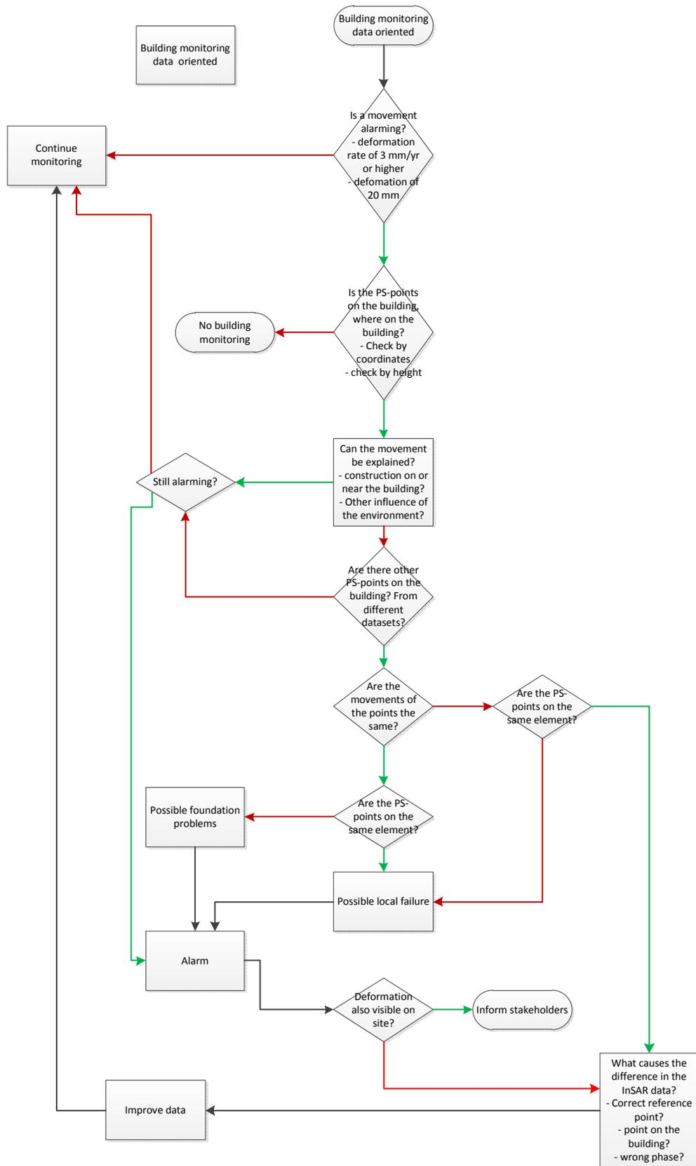
Figure 5.17, the decision tree for using InSAR in data-oriented building monitoring. Diamond shapes are decisions, rectangle a process, red arrows are negative and green arrows are positive.
