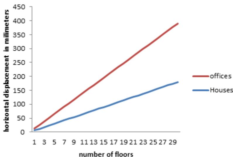
Figure 4.23, Graph of maximum horizontal displacement, according to Eurocode limits.
