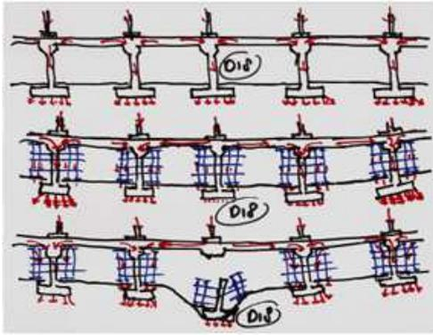
Figure 5.28, schematic presentation of the development of the sag of the column. Source: Dossier Hageman 7998 sinkhole winkelcentrum 't Loon in Heerlen, 2012.
