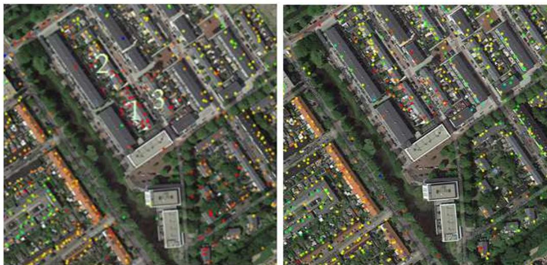
Figure 5.10, descending data of the Goudenregenlaan can be seen in the left figure and ascending data in the right of the TerraSAR-x satellite. The buildings with large deformations are numbered. The data is provided by Hansje Brinker. The data of Delft is recorded with the TerraSAR-x satellite and projected on Google Maps. The original scale is approximately 1:2500 (edited images).
