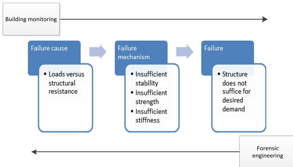
Figure 4.1, Workflows of the different disciplines. With building monitoring, changes in the behaviour of a structure are monitored. Forensic engineering researches the cause of failure.
