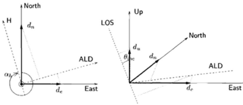
Figure 2.7, Projection of the three components of the deformation vector (Up, East, and North) onto the satellite line-of-sight (LOS). The left figure shows the top view, showing the North and East components on the azimuth look direction (ALD), which is perpendicular to the satellite's heading (H). The heading angle is indicated by  $\alpha_h$ . The right figure includes the projection of the Up component to the LOS via incidence angle  $\theta_{inc}$ . Source: Hanssen (2001)
