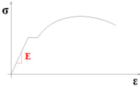
Figure A2.3, a stress-strain diagram of steel. Marked in red is a part of the linear range of the stress-strain diagram. This can be expressed as the Young's modulus.
