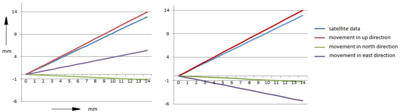
Figure 4.6, Red indicates the measured satellite data, and blue, green, and purple indicate movement, if it is assumed that the point does not move in any other direction. The right figure shows ascending data, and the left figure shows descending data.
