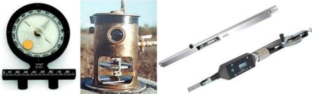
Figure 4.4, Examples of, from left to right: inclinometer, tiltmeter, electrolevel beam, and a tape extensometer. Source: <http://www.wikipedia.org>.
