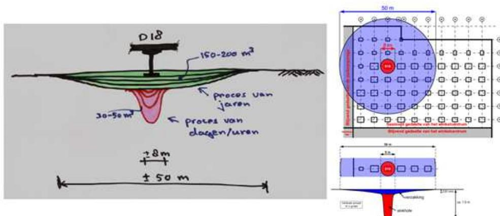
Figure 5.27, right: sketch of the subsidence of the column in time and left: the area around the column that sagged. Source: Dossier Hageman 7998 sinkhole winkelcentrum 't Loon in Heerlen, 2012.
