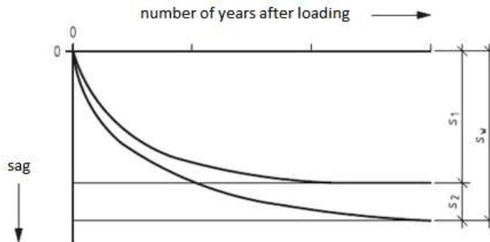
Figure 4.17, Consolidation process of a raft foundation over time. Source: Eurocode NEN-EN 9097 (2012)
