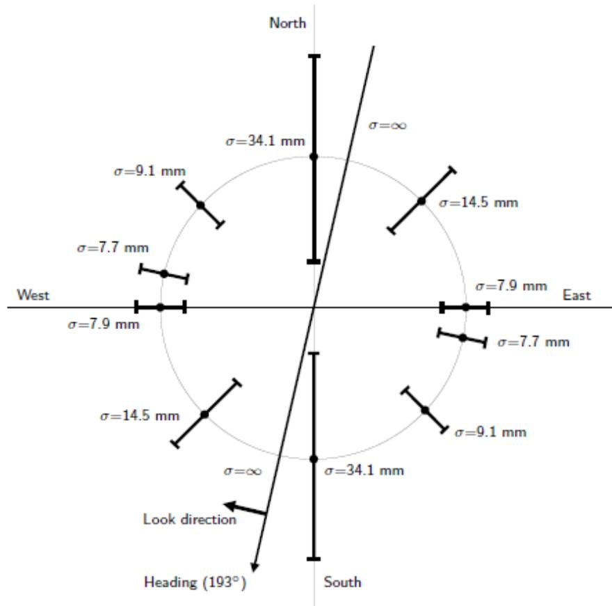
Figure 2.11, Insensitivity for displacement in the North direction. A standard deviation of 34.1 mm can be expected, when a standard deviation of 3 mm in the LOS direction is assumed for the Envisat satellite. (Leijen, 2014)
