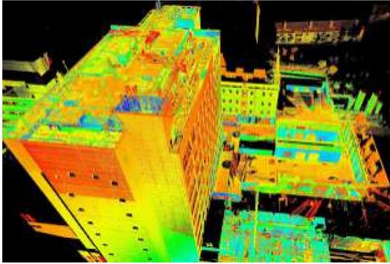
*Figure 4.3, Lidar data in a Revit BIM model. Source: <http://severnpartnership.blogspot.nl/2011/09/laser-scan-to-3d-revit-bim-model.html>*
