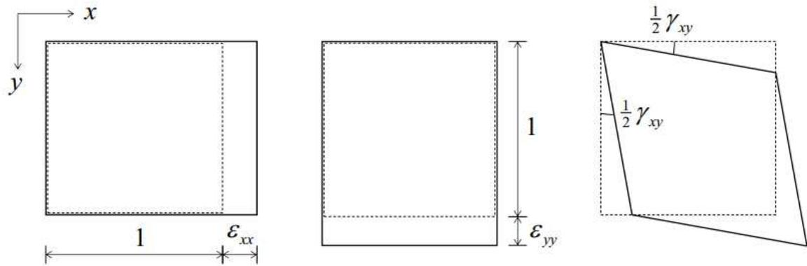
Figure 4.9, Different deformations of an element. Source: Lecture notes plates and slabs (2011)
