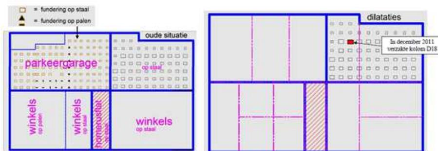
Figure 5.26, the floor plan of the structure with dilatations. Source: Dossier Hageman 7998 sinkhole winkelcentrum 't Loon in Heerlen, 2012.
