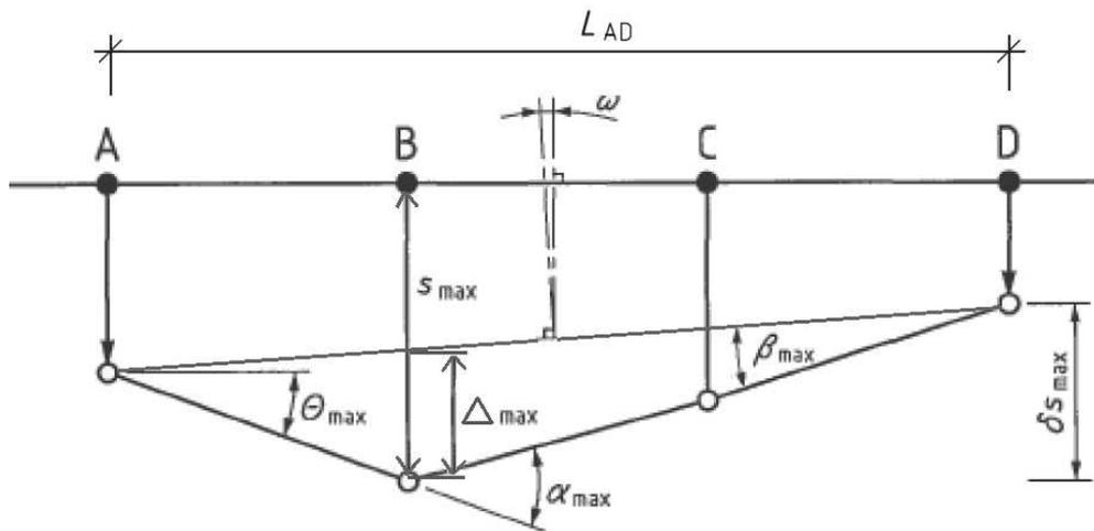
Figure 4.25, Different deformation parameters for a foundation, according to the Eurocodes and other research.
