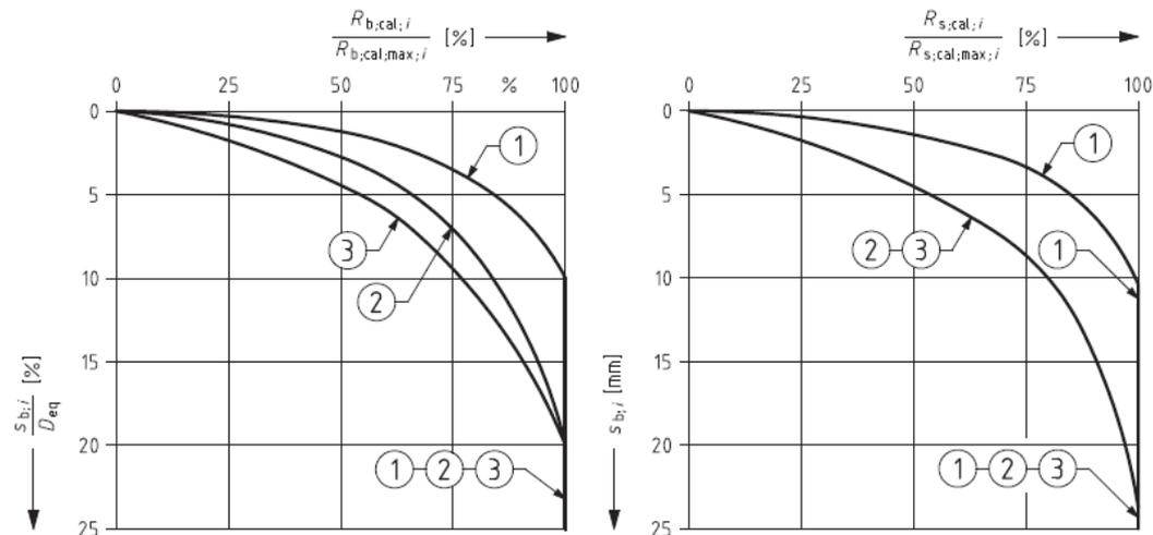
Figure 4.19, The value  $s_b$  can be determined with the graphs. NEN 9097-1 (2012)
