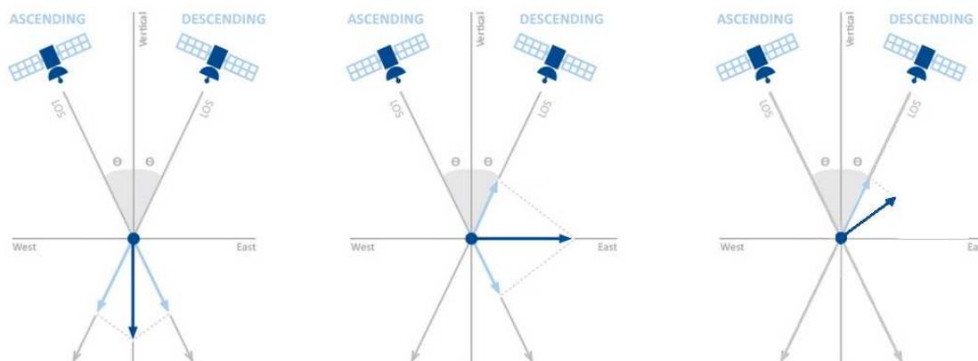
Figure 2.13, The difference between ascending and descending data for the Up and East direction. The dark blue arrows are the direction of movement of a PS-point, while the light blue lines are the information recorded by the satellite for different tracks. (TRE website)
