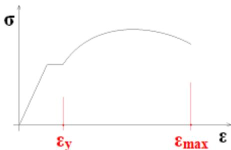
Figure A2.4, a stress-strain diagram of steel. Marked between the red dots is the ductility.
