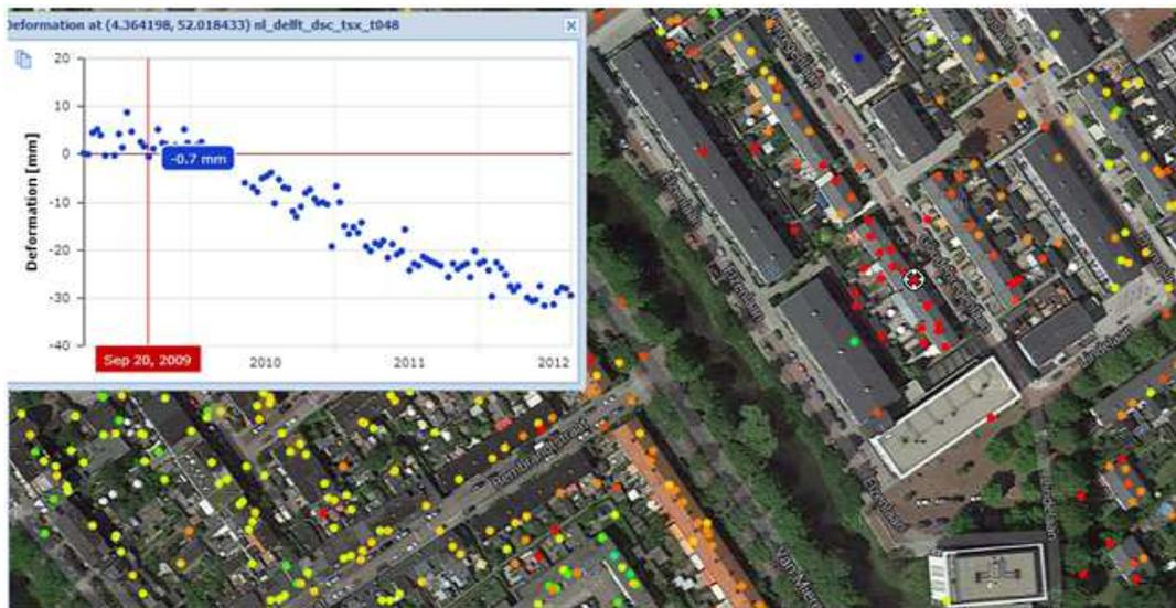
Figure 5.13, deformation development of the white marked point on building 1. The deformation started at the same time as the construction in the end of September 2009. The data of Delft is recorded with the TerraSAR-x satellite and projected on Google Maps. The original scale is approximately 1:1333 (edited images).
