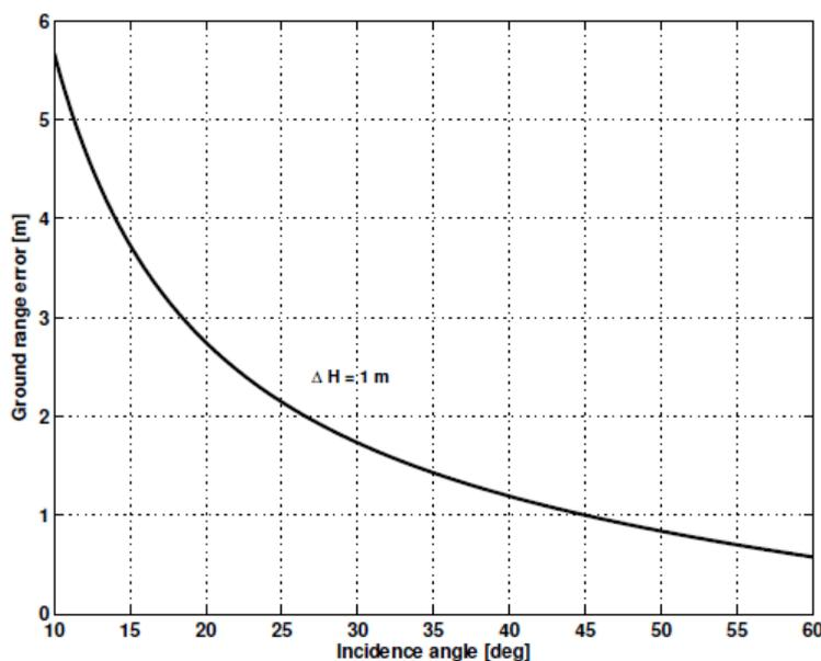
Figure 2.5, Geolocation error in ground range (m) due to height error of one metre. The error is dependent on the incidence angle. Source: Van Leijen (2014).
