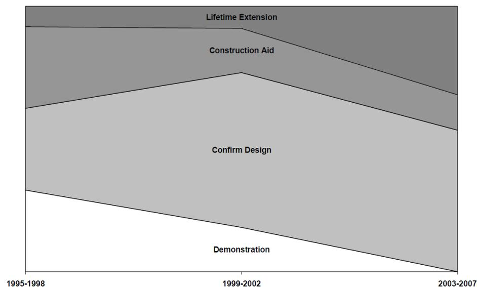
Figure 4.2, Reasons for monitoring bridges. Source: Inaudi (2008), Overview of 40 Bridge Structural Health Monitoring Projects.
