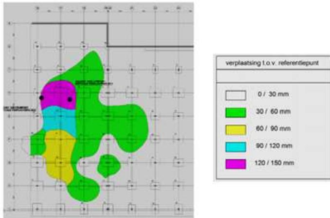
Figure 5.29, the movement of the parking floor according to Dossier Hageman 7998 sinkhole winkelcentrum 't Loon in Heerlen, 2012
