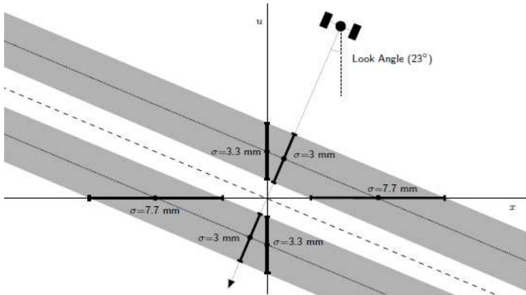
Figure 2.8, Sensitivity of a satellite (Envisat) in the Up and East direction. (Van Leijen, 2014)
