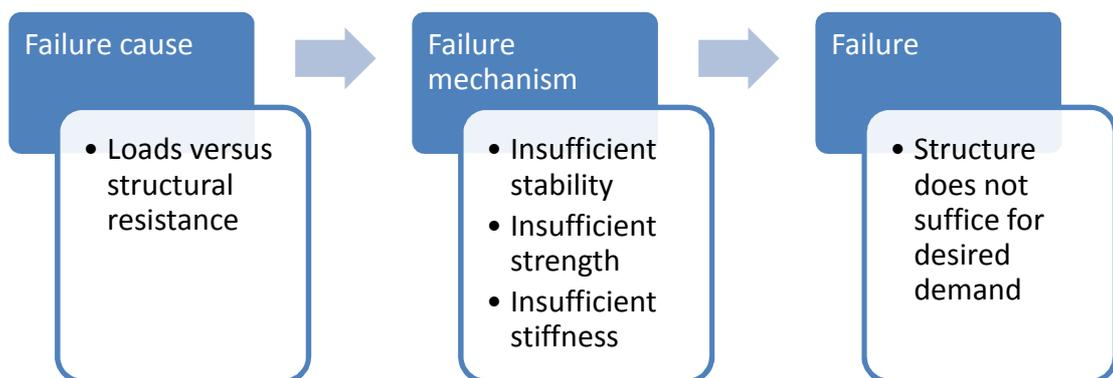
Figure 3.1, The cause of failure.
