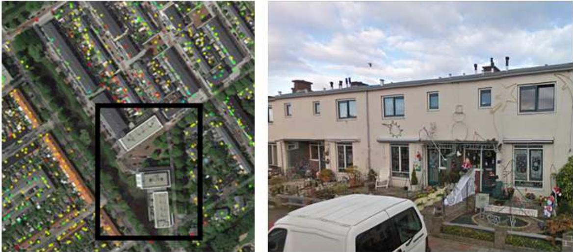
*Figure 5.11, building that lacks PS-points in the left image. This can mean no stable points can be found in this area, because of construction activities. The data is provided by Hansje Brinker. The data of Delft is recorded with the TerraSAR-x satellite and projected on Google Maps. The original scale is approximately 1:2500 (edited images). In the right figure a Google Maps street view of the houses at the Goudenregenlaan.*
