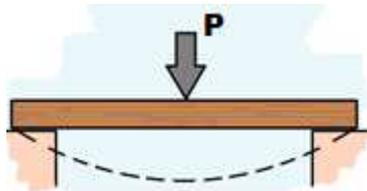
Figure A2.2, example of possible deflection of wooden beam as dotted line.
