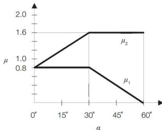
Figure 4.12, Snow load shape coefficient. Source: NEN-EN 1991-1-3 (2011)
