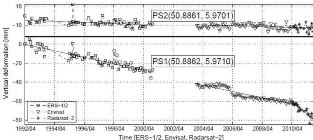
Figure 5.37, the deformation of the two PS-points in time monitored by different satellites. Source: Detection of cavity migration and sinkhole risk using radar interferometric time series by Chang en Hanssen (2014).
