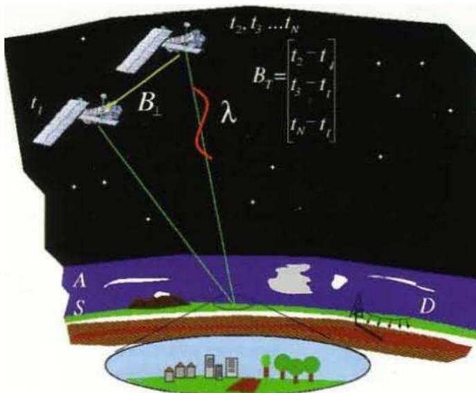
Figure 2.2, Design parameters of InSAR. Source: (Hanssen et al. 2002) Design Parameters and Environmental Factors Affecting Feasibility Deformation Monitoring by Satellite Interferometry
