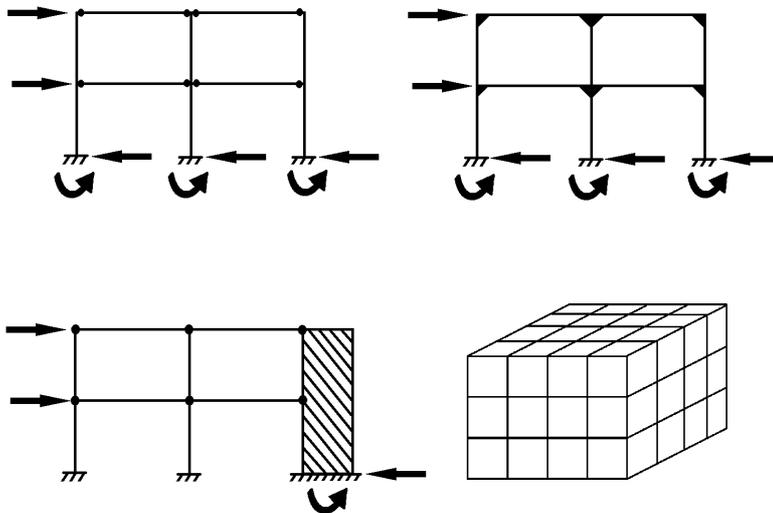
*Figure A2.8, different stability systems, from left to right: column fixed to the foundation, moment resisting frame, shear walls or shear cores, fixed to the foundation and load bearing facades.*
