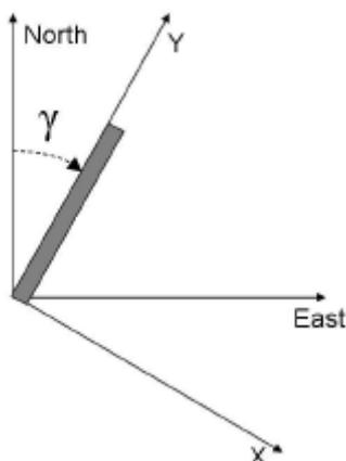
Figure 2.9, Transformation of the coordinate system from global to local.
