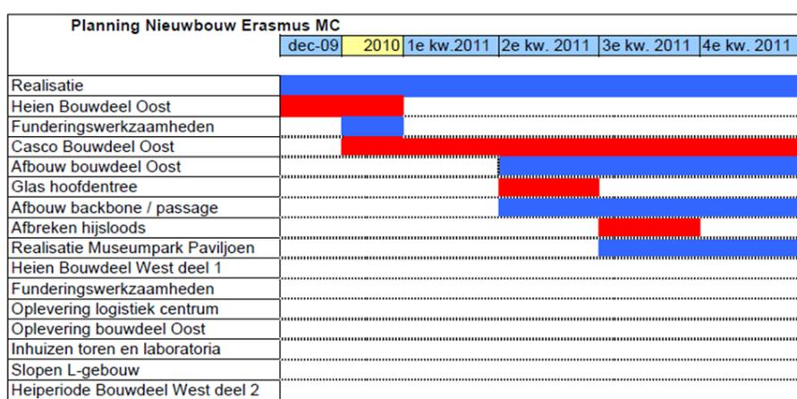
Figure 5.22, planning of construction activities for the eastern part of the new high-rise. Source: [Erasmusmc.nl/nieuwbouw](http://Erasmusmc.nl/nieuwbouw).
