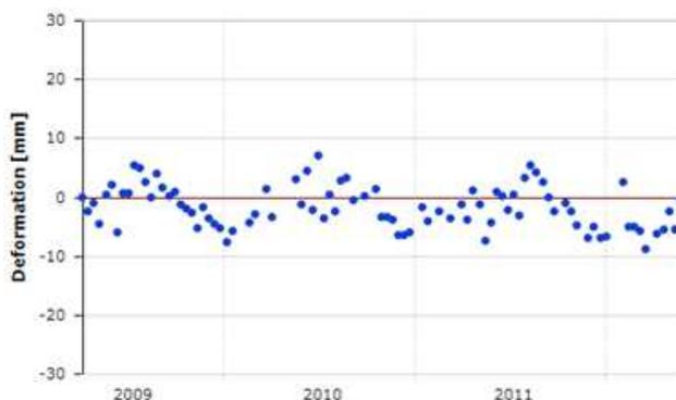
Figure 5.19, deformation data of Erasmus MC from April 2009 until May 2012 monitored with TerraSAR-x, data provided by Hansje Brinker.
