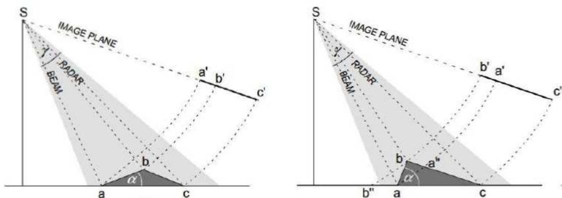
Figure 2.4, Foreshortening can be seen in the left figure. The slope of hill a-b is represented as shorter than it is in reality. Layover can be seen in the right figure. Due to the steep slope and the height of hill a-b, the hill is presented incorrectly in the data. (Olmsted, 1993)
