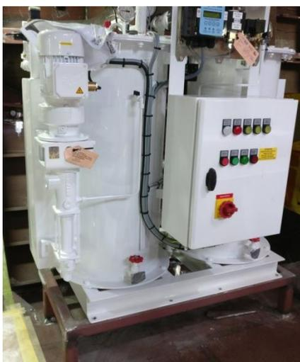
Figure 3 Modular oil-water separator
