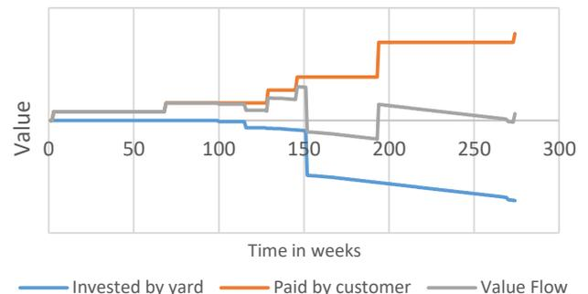
Figure 1 the value time curve of the current engine room assembly process
