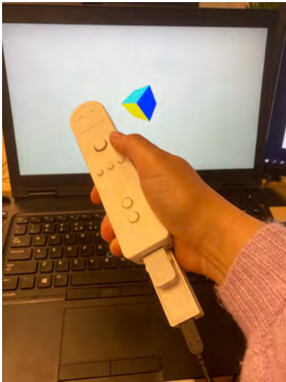
Figure 4.2: The orientation of the Voodoo Doll is visualized with a colored cube.
